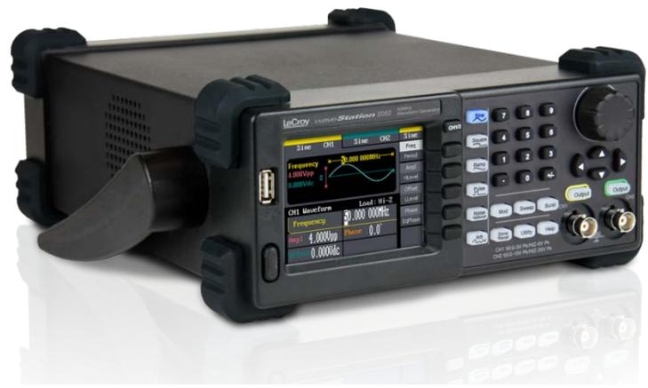
**Figure 1: Shown is LeCroy’s WaveStation 2052 function/arbitrary waveform generator, which sports a bandwidth of 50 MHz, a 125-Msample/sec sampling rate, 14-bit resolution, and 16 kpoints of memory per channel**
