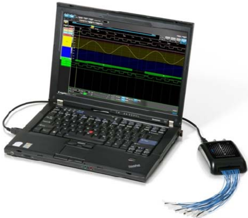
Figure 1: Shown is LeCroy's LogicStudio 16-channel logic analyzer, which links to a PC running the companion LogicStudio software
