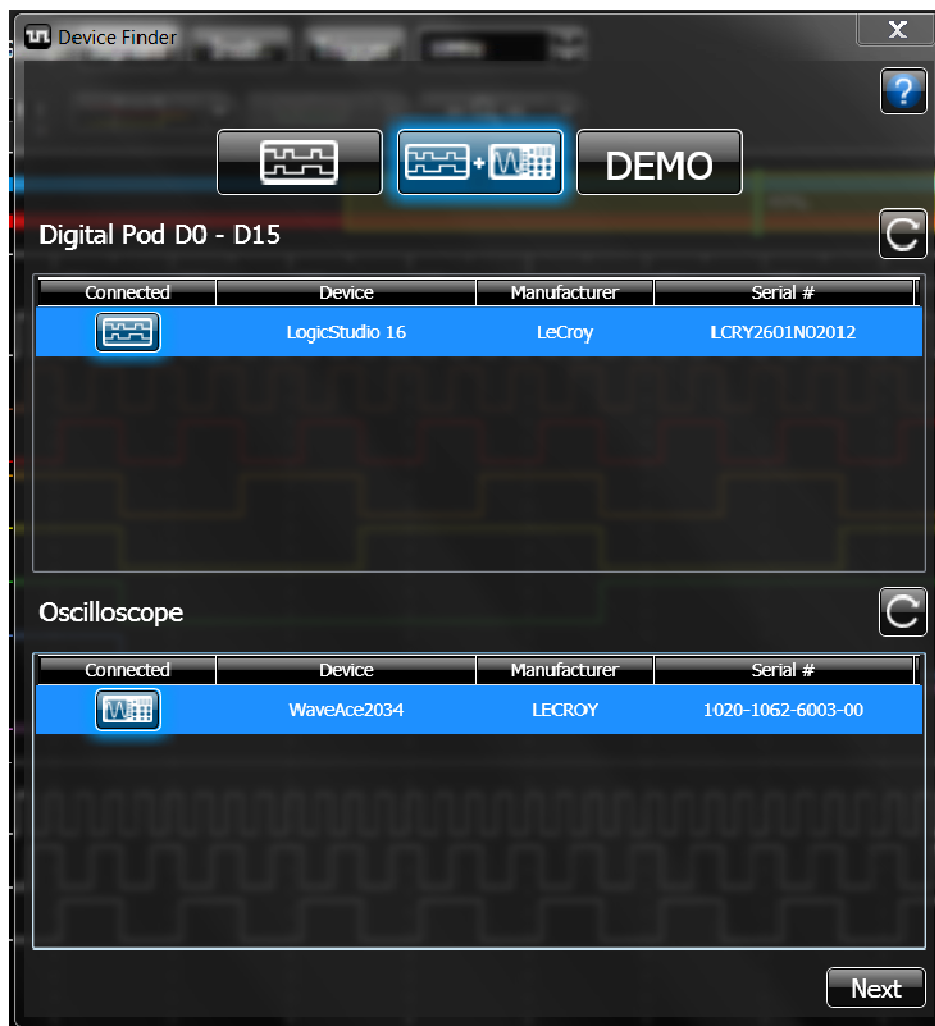
Figure 3: LogicStudio's Device Finder wizard facilitates USB connection of the LogicStudio logic-analyzer module and the WaveAce oscilloscope to the PC
