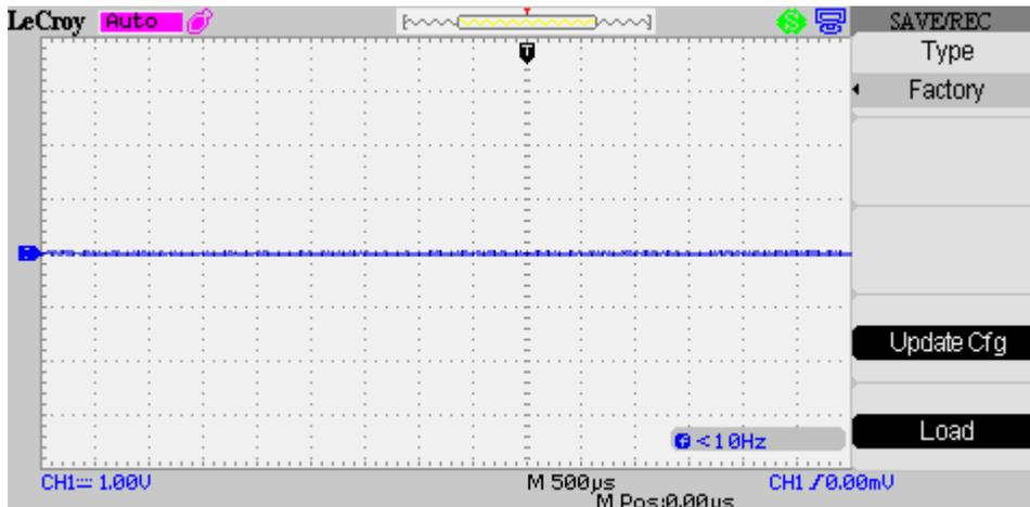
At any time the menu on the right-hand side of the screen can be removed/restored by pressing the front panel MENU ON/OFF button.
