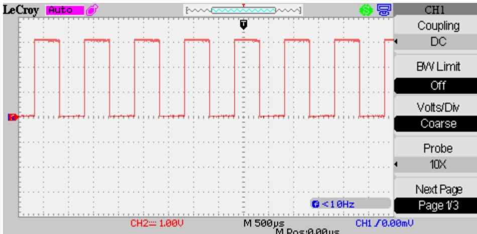
**Step 3:** Press the SAVE/RECALL button. Select Type as Setup, Save To as Device and Setup to No. 1. Now press the menu Save button.
