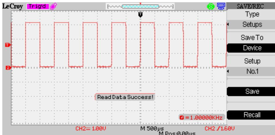
To prevent the trace being overwritten the scope is switched to Stop mode. Reconnect the probe and press RUN/STOP to restart the acquisition.
