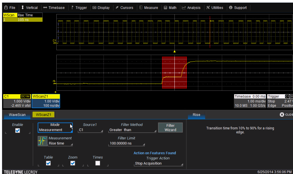
Figure 2: Here, WaveScan has found the glitch it was seeking in the input signal
