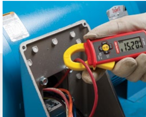
Utilize the inrush current function for motor start-up monitoring.
