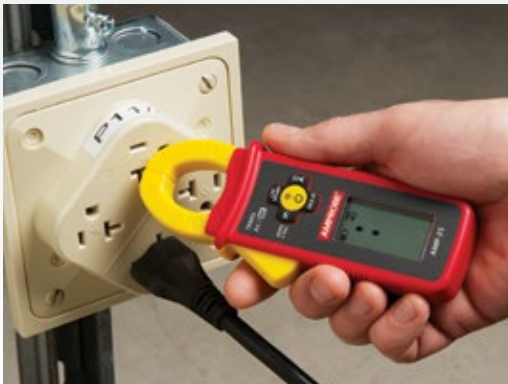
The non-contact voltage (NCV) function checks for voltage presence.
