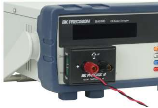
Connected to external DC source supplying 5 V and 3 A
