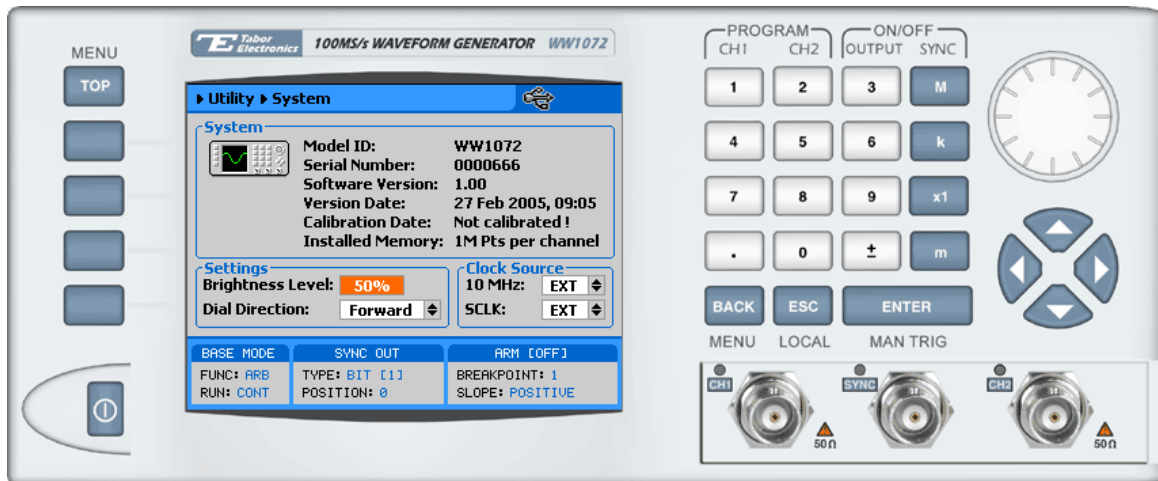
Figure 3-15, Modifying the SCLK and 10MHz Clock Source
