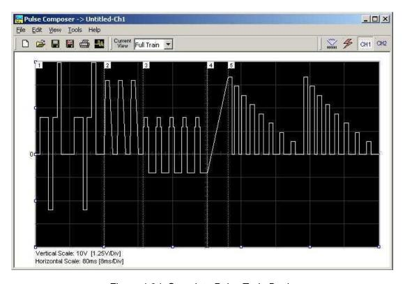
Figure 4-34, Complete Pulse Train Design
