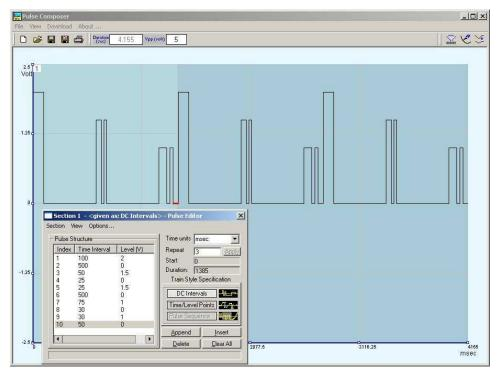
Figure 1-5, ArbConnection – The Pulse Composer
