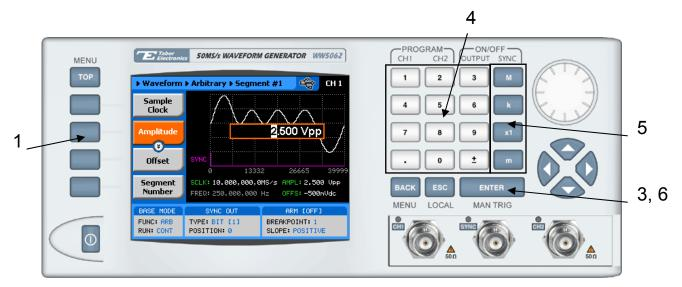
Figure 3-8, Programming Amplitude and Offset
