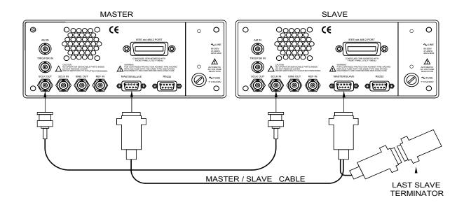
Figure 3-29, Wiring Diagram Master to Slave
