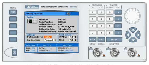
Figure 3-15, Modifying the SCLK and 10MHz Clock Source
