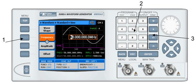
Figure 3-5, Modifying Output Frequency
