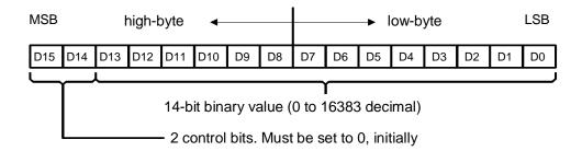
Figure 5-2. 16-bit Initial Waveform Data Point Representation
