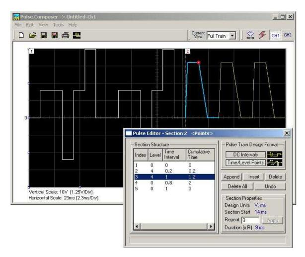
Figure 4-39, Building Section 2 of the Pulse Example
