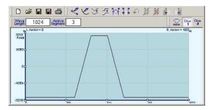
Figure 1-10, Segment 3 - Pulse Waveform
