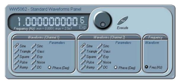
Figure 4-4, The Standard Waveforms Panel
