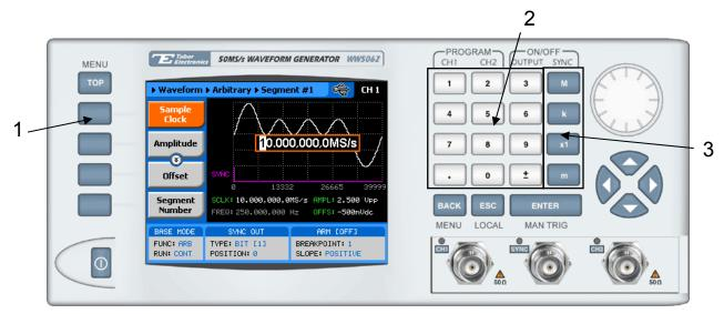
Figure 3-6, Modifying Sample Clock Frequency
