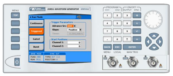
Figure 3-10, Trigger Run Mode Parameters
