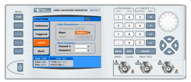
Figure 3-11, Gated Mode Parameters
