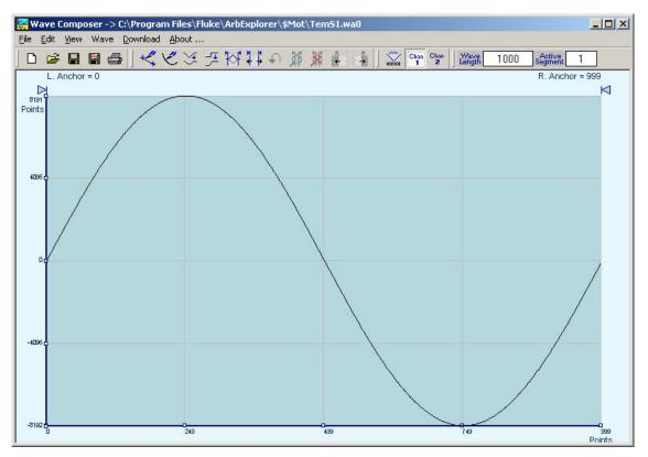
Figure 4-15, The Wave Composer Opening Screen
