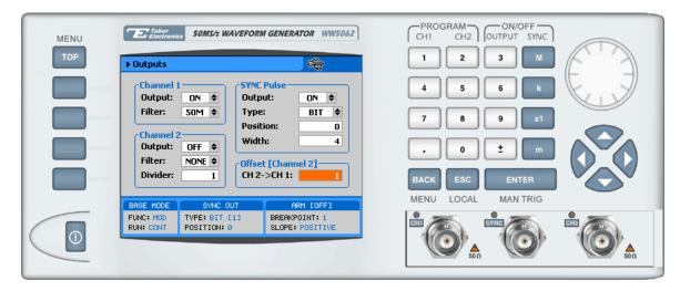
Figure 3-28, Adjusting Phase Offset Between Channels
