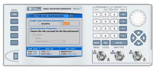
Figure 3-30, Setting up Master/Slave Parameters
