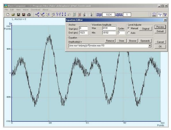
Figure 4-29, Combining Waveforms into Equations
