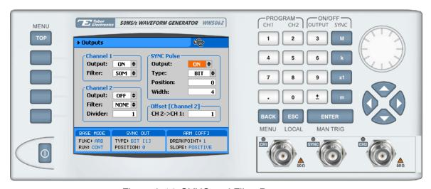
Figure 3-14, SYNC and Filter Parameters
