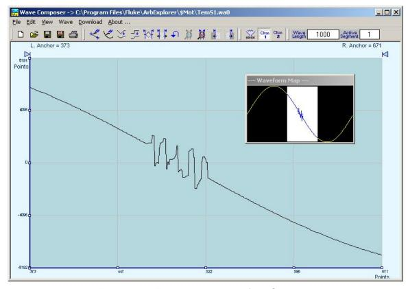
Figure 4-17, Zooming In on Waveform Segments
