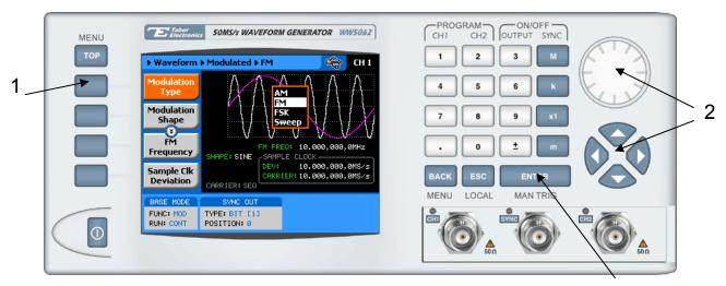
Figure 3-22, Selecting a modulated Waveform
