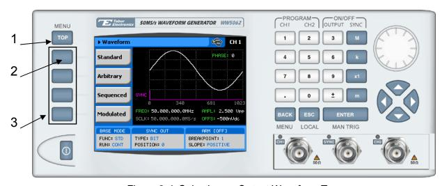
Figure 3-4, Selecting an Output Waveform Type
