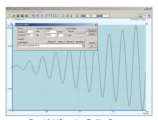
Figure 1-3, ArbConnection – The Wave Composer
