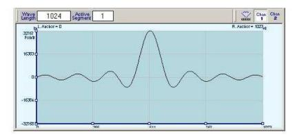
Figure 1-8, Segment 1 – Sin (x)/x Waveform
