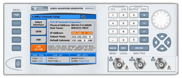
Figure 2-11, LAN Configuration Screen
