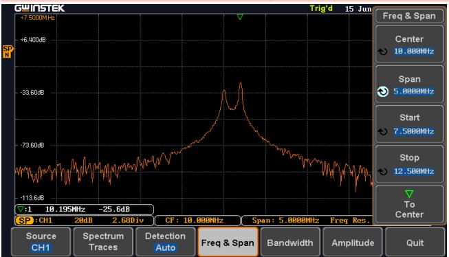
The input signal is FSK  $500mV_{pp}$  sine wave
