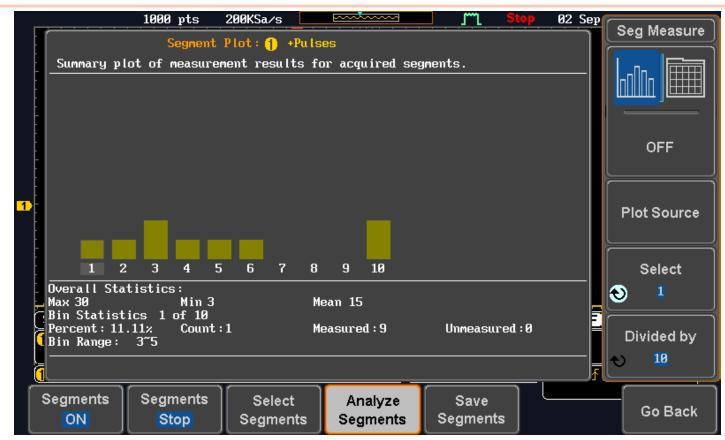
•Available to analyze the value of Max ,Min ,Mean data of the segmented memory.
