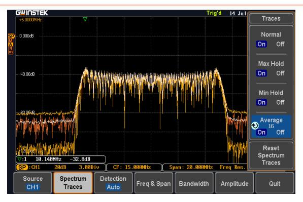
In order to allow users to experience genuine Spectrum Analyzer, MDO-2000E also includes Spectrum Trace Type settings (Normal, Max-hold, Min-hold, and Average). Users can freely simultaneously select various Spectrum Traces.
