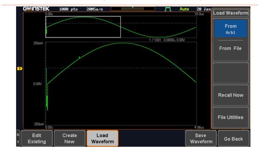
User is allow to load and create arbitrary waveform on the MDO-2000E series .
