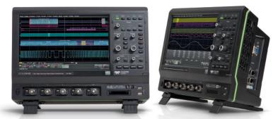
HD06000 uses Teledyne LeCroy's HD4096 high definition true 12-bit technology, long memory, a compact form factor, 12.1" touch screen display, powerful measurement and analysis tools, and mixed signal capability. It is the ideal oscilloscope for circuit validation, system debug and waveform analysis.
