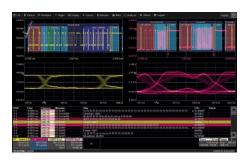
WaveRunner 8000 combines Serial Bus Trigger, Decode, Measure/Graph, and now also Eye Diagrams
