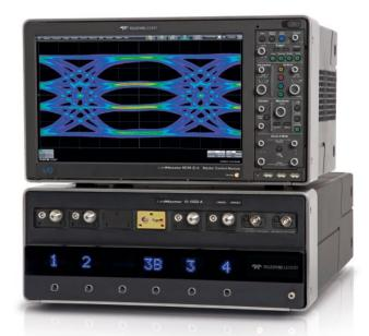
The LabMaster 10 Zi-A series of real-time oscilloscopes boasts the world's highest bandwidh and fastest sampling rate at 100 GHz and 240 GS/s. This world-leading performance is key to acquiring, analyzing and understanding the fastest phenomena found in R&D labs, where engineers are working on next-generation communication systems, high bandwidth electrical components and fundamental scientific research.
