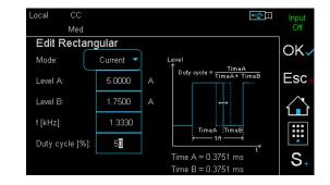
With the PWM function, the switching frequency and the duty cycle can be set for the two amplitude values in manual operation.
