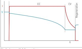
The discharge function tests energy storage devices such as batteries, ultracaps and electrolytic capacitors etc. by discharging them in CC, CP or CR mode. The discharge function can be combined with the list function so that pulsed discharge is possible.
