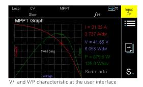
The Maximum Power Point Tracking (MPPT) function consists of the two sub-functions Sweeping and Tracking, which alternate continuously in an adjustable interval.
