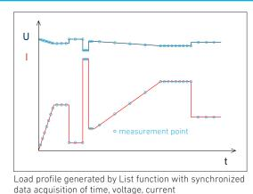
In all operating modes CC, CV, CR, CP the electronic loads can produce load profiles by List function. Up to 300 settings with variable dwell and ramp times are possible.
