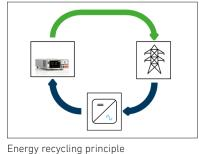
The absorbed power is fed back into the mains supply<sup>1)</sup>. This alone reduces electricity costs, and the environment is only minimally heated. Powerful fans are not required for regenerative loads, which makes the devices pleasantly quiet compared to linear loads and thus perfect for laboratory operation.
