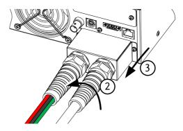
4. Remove the AC power cord wires.
