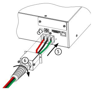
7. Turn the power on. The AC power supply is now ready to power the DUT.
