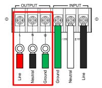
APS-7100 shown. The input terminals are already connected and shows which output terminals are to be connected.
