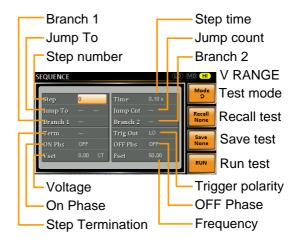
Sequence Parameter Overview The Sequence function is comprised of a minimum of 2 steps that are executed in user defined sequences.
