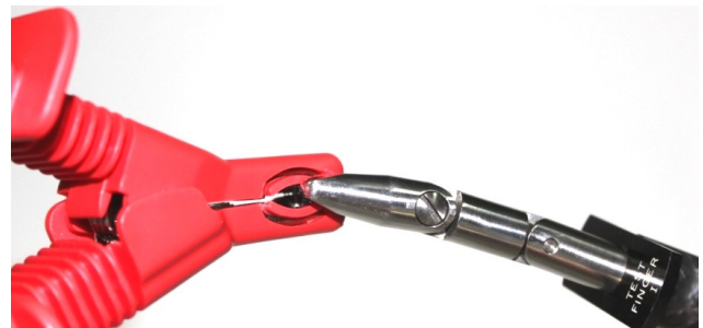
Megger test clip being tested with a IEC standard test finger for creepage and clearance
