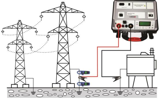
Figure 1: GGT500 cable connection for ground grid test
