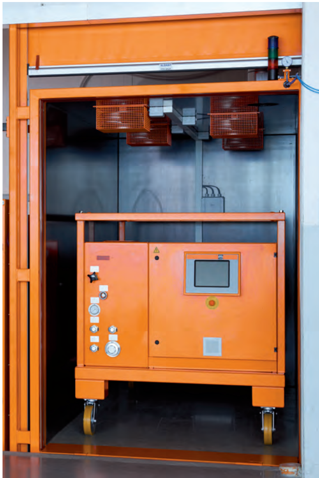
Atmospheric test chamber with automatic roller shutter
