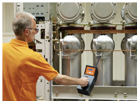
The SF 6 LeakSpy allows the detection and quantification of smallest SF 6 concentrations (indication accuracy: 1 ppm v )
