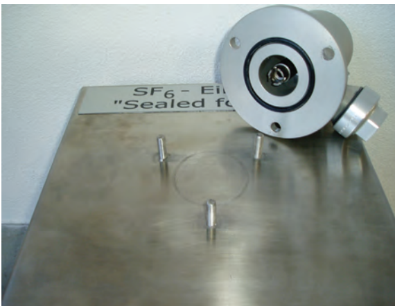
Fixation of welded stud before assembly on surface
