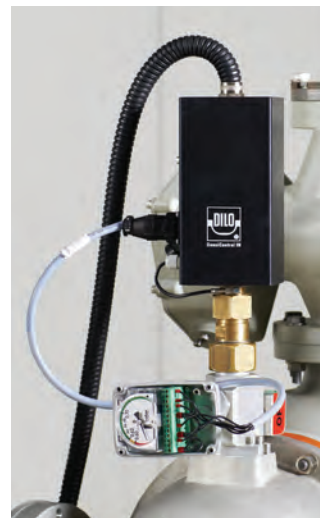
Connecting box of density monitor in assembled condition
