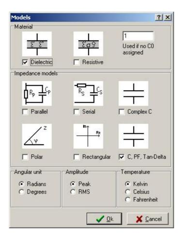
Selected models appear at the bottom of Results window, where one can choose which parameters are to be shown. Below the Dielectric and C, PF, Tan-Delta models are chosen to be used in Results and  $\epsilon'$  as a parameter is displayed in the graph.
