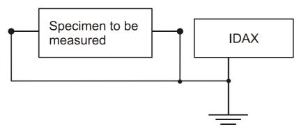
2. In the case of Test Capacitor, keeping the electrodes grounded while connecting IDAX leads is complicated. Therefore, in this particular case with Test Capacitor, it is permitted to remove the ground connections before connecting IDAX.
