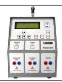
Generates 10 V to 300 V DC on coils outputs.
