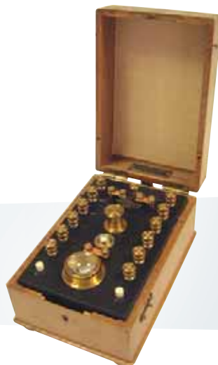
This calibration potentiometer dating from 1900 was used with a standard battery and a galvanometer like the one shown above. Its price was 195 francs!
