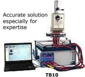
Three phase fully automated 0.02 or 0.05 accuracy class test station for electricity meter testing up to 120A.
