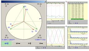
Verification of power network wiring in "star" and "delta" connection – graphical display of three phase voltage and current vector and direction of vector rotation.
