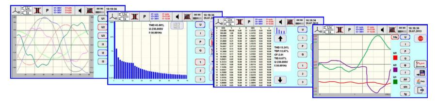
▶ measuring of power quality parameters according to IEC 61000-4-30 class A with visualization of measurement results in the real time mode
