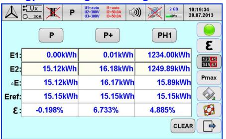
function of energy measurement with method of setting time periods for verification of energy meter Register directly in percent [%],
