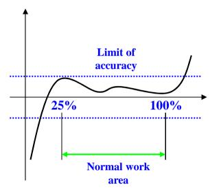
CT – current transformer can operate with stated accuracy only between 25% - 100% of burden (load). In case of too long, or too thin wire dimension or too small load, the result, secondary current can be out of accuracy limits
