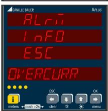
Alarm display: By shortly pressing the key an operating mode is started, which allows to display alarm state texts and to acknowledge alarms via line 4. If there are no configured alarms the message "No LED used" is displayed and then the mode is stopped. Otherwise the mode is automatically stopped after 30s without any key pressed or via the key. If this mode is active no measurement info is displayed on line 1 to.
