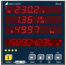
**Measurement display:** Is the normal operating mode of the device. By means of the navigation keys different measurement display can be selected. Depending on the selected display mode and the system monitored different measurement displays are available.
