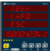
**Meter reading**: By pressing the key **i** for a longer time an operating mode is started, which allows to read all the meter contents via line 4. This mode is automatically stopped after 30s without any key pressed or via the key **c**. If this mode is active no measurement info is displayed on line 1 to 3.
