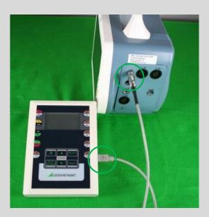
Connection of temperature test cable and SECULIFE NIBP for measuring the temperature, a standard temperature test cable is connected between SECULIFE NIBP and the DUT.
