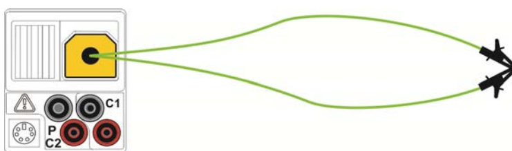
Figure 5.10: Shorted test leads
