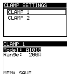
Figure 4.9: Configuration of current clamp measuring inputs
