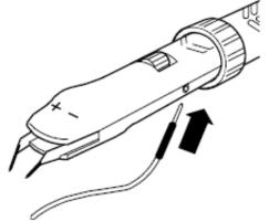
Connect the plug of the ground lead to the receptacle located on the side of the amplifier/adjustable tip module body.
