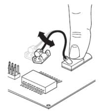
Applying pressure when adjusting the probe holder
