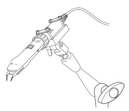
Attach the probe by first removing the screws holding the top plate to the V-shaped probe holder. Insert the end of the platform/cable assembly and tighten the screws holding the top plate to secure the probe.
