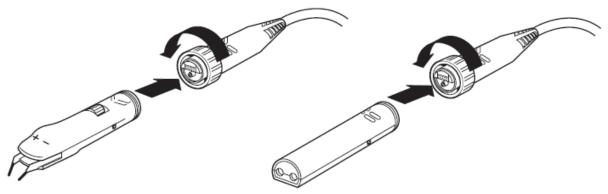
Attaching Adjustable Tip or Amplifier Module
