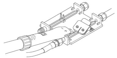
Adjustable Tip module connected to PCF200
