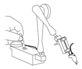
Attach the probe by first removing the screws holding the top plate to the V-shaped probe holder. Rest the Long Interconnect Extender in the V-shaped groove, and fasten the top plate to the holder, using the removed screws (as follows). Then, insert the Dx10 or Dx20-PT onto the Long Interconnect Extender.
