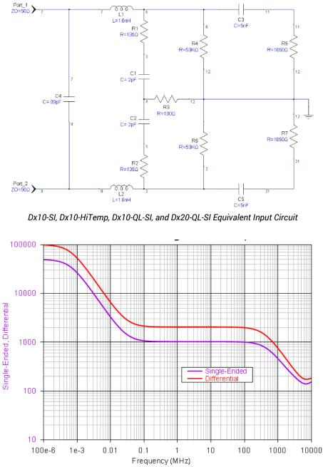
Dx10-SI, Dx10-HiTemp, Dx10-QL-SI, and Dx20-QL-SI Single-ended Impedance
