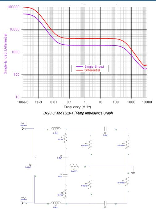
Dx20-QC Equivalent Input Circuit
