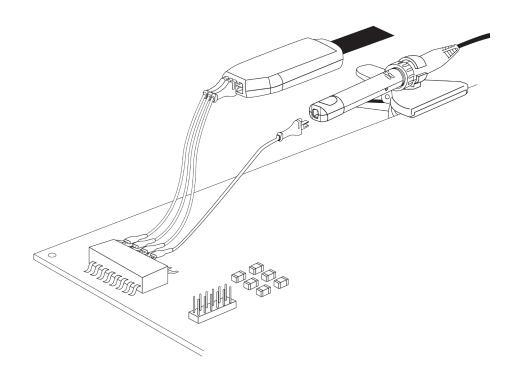
Switching QL-SI tips between WaveLink probe and HDA125
