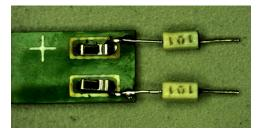
2. Bend the tips in toward the center. Make the bend as close to the resistor body as possible. Bend them to about 60° from straight.
