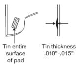
4. Locate the socket so the closed end is slightly overhanging the end of the pad. This prevents solder from flowing into the socket insert hole. Align the socket sides with the pad sides and solder as shown. Leave proper clearance between the socket and pad sides when soldering.
