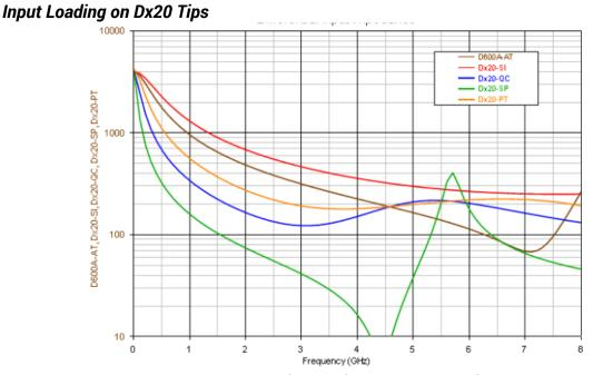
Dx20 SI/QC/SP/PT/HiTemp and D600A-AT Input Impedance
