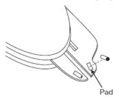
3. Tin the pad using a no clean solder (shown below). Tin thickness should be .010" to .015" (2.5 to 4 mm).
