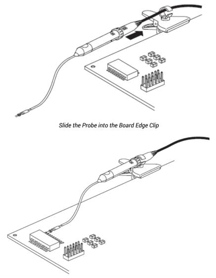
Insert the probe body into the board edge clip and position the clamp as desired.
