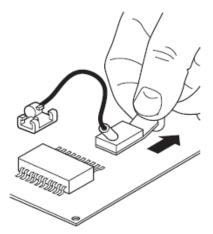
Removing the Retaining Clip
