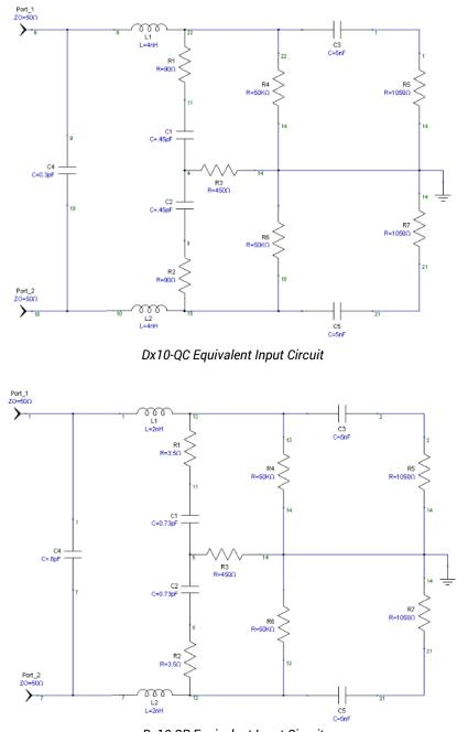
Dx10-SP Equivalent Input Circuit
