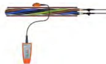
For an even safer selection, this system provides the possibility to use the Flex Coupler to select the correct cable first and then to confirm this additionally by using the twist field
