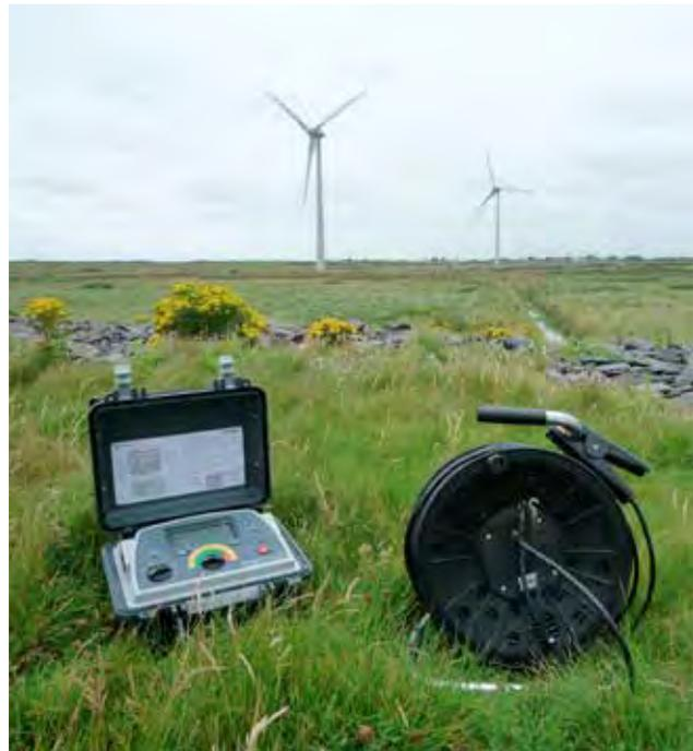
KC test leads used with a DLR010 HD for testing continuity of wind turbines
