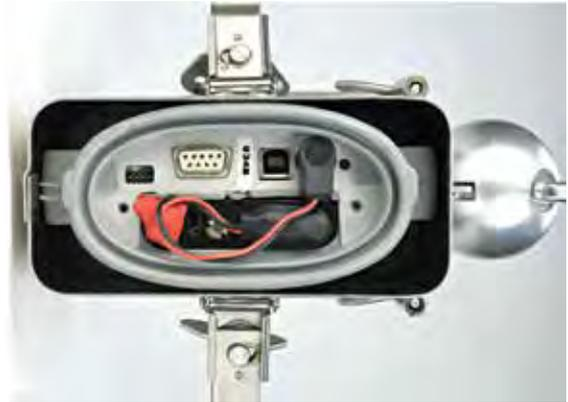
Easy plug-in access allows for quick data retrieval via RS-232 and USB cable ports. The battery compartment is specifically designed for simple removal and installation.
