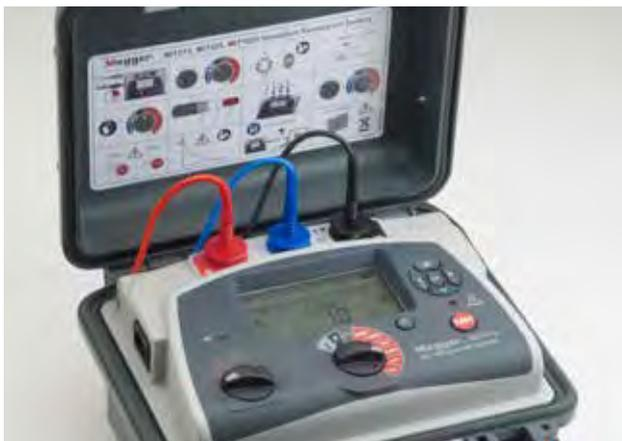
The new MIT1515 is lighter and has instantly swappable batteries
