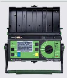
A broad-range measuring device allows for use of the test instrument in all alternating and 3-phase electrical systems with voltages from 65 to 500 V and frequencies of 15.4 to 420 Hz
