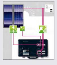
Connect ○ Switch On ○ Start Measurement ○ Read Results ○ Done!
