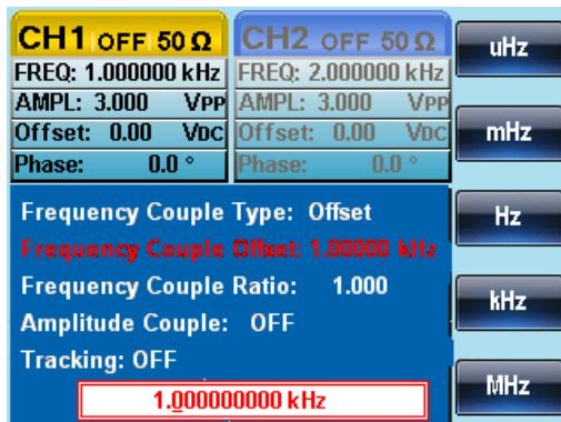
5. Change the frequency coupling mode to Ratio. Set the ratio to 2.
