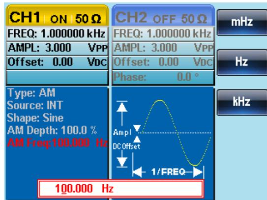
5. Use the arrow keys and scroll wheel or number pad to enter the AM frequency.
