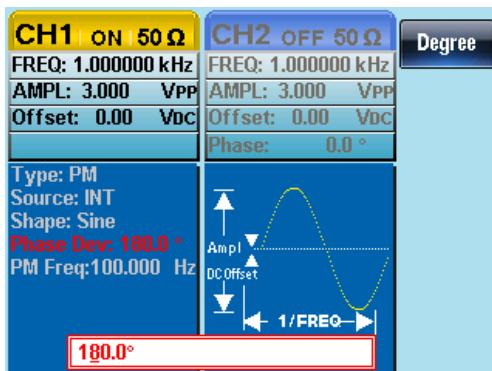
5. Use the arrow keys and scroll wheel or number pad to enter the phase deviation.
