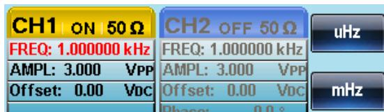
3. Use the arrow keys and scroll wheel or number pad to enter the carrier frequency.
