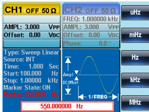
7. Use the arrow keys and scroll wheel or number pad to enter the frequency.
