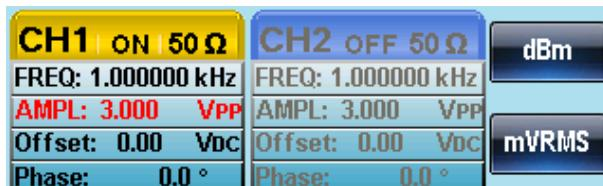
3. Use the arrow keys and scroll wheel or number pad to enter the amplitude.
