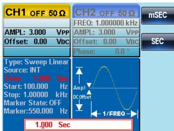
5. Use the selector keys and scroll wheel or number pad to enter the Sweep time.
