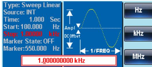
4. Use the arrow keys and scroll wheel or number pad to enter the Stop/Start frequency.
