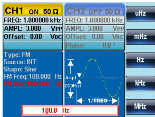
5. Use the arrow keys and scroll wheel or number pad to enter the frequency deviation.
