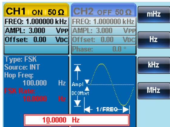
5. The arrow keys and scroll wheel or number pad to enter the FSK rate.
