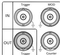
Marker output signal. Used for Sweep and ARB mode only.
