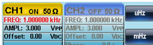
3. Use the arrow keys and scroll wheel or number pad to enter the frequency.
