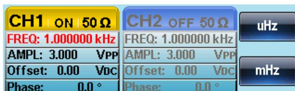
3. Use the arrow keys and scroll wheel or number pad to enter the frequency.
