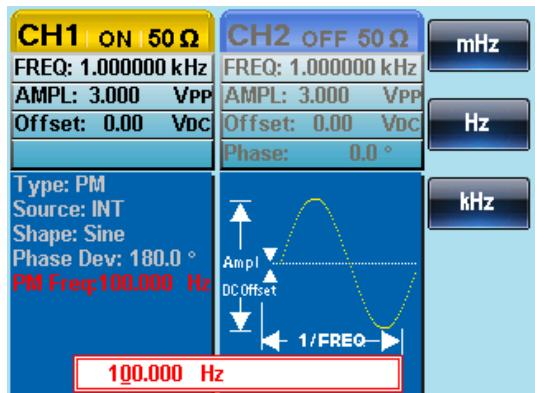
5. Use the arrow keys and scroll wheel or number pad to enter the PM frequency.
