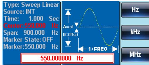
5. Use the arrow keys and scroll wheel or number pad to enter the Span/Center frequency.
