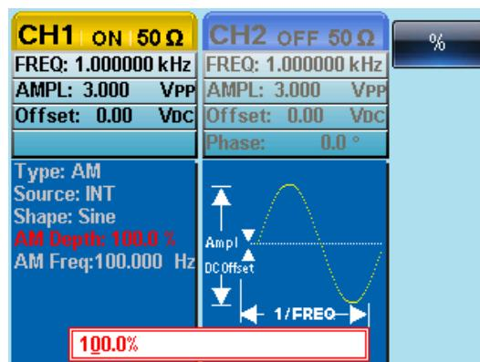
5. Use the arrow keys and scroll wheel or number pad to enter the AM depth.
