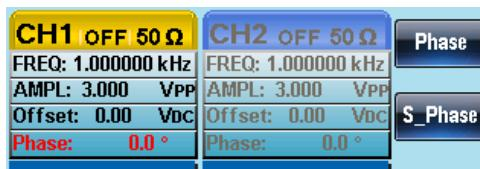
4. Use the arrow keys and scroll wheel or number pad to enter the output phase.
