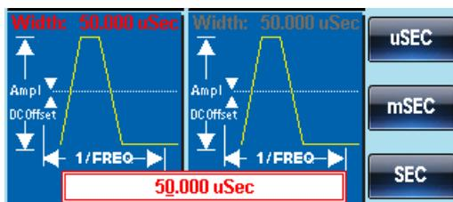
4. Use the arrow keys and scroll wheel or number pad to enter the pulse width.
