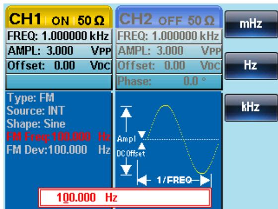
5. Use the arrow keys and scroll wheel or number pad to enter the FM frequency.
