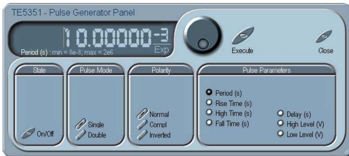
Figure 3-20, the Digital Pulse Generator Panel
