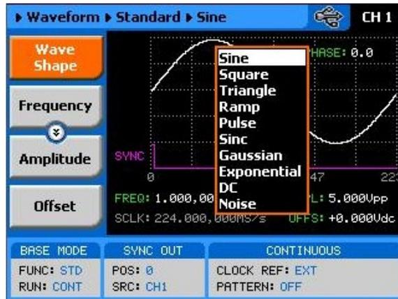
Figure 3-46, Built-in Standard Waveforms Menu
