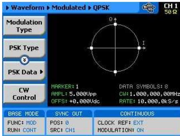
Figure 3-74, PSK Modulation Display Example
