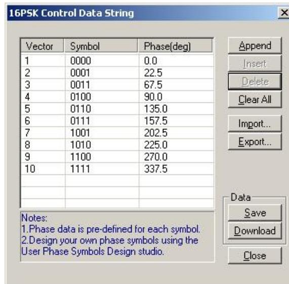
Figure 4-21, 16PSK Data Table Sample
