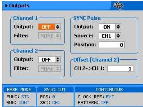
Figure 3-97, Programming Phase Offset between Channels
