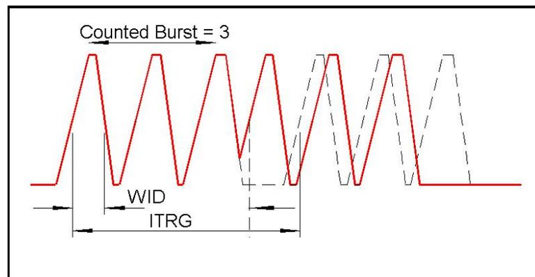
Figure 3-45, Output Waveform with Error 108 (208) Example
