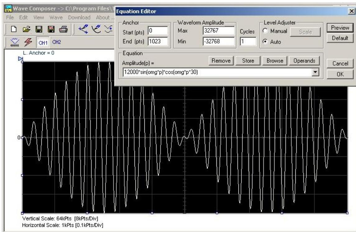
Figure 4-42, Using the Equation Editor to Modulate Sine Waveforms.
