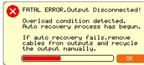
Figure 3-1, Auto Recovery from Overload conditions
