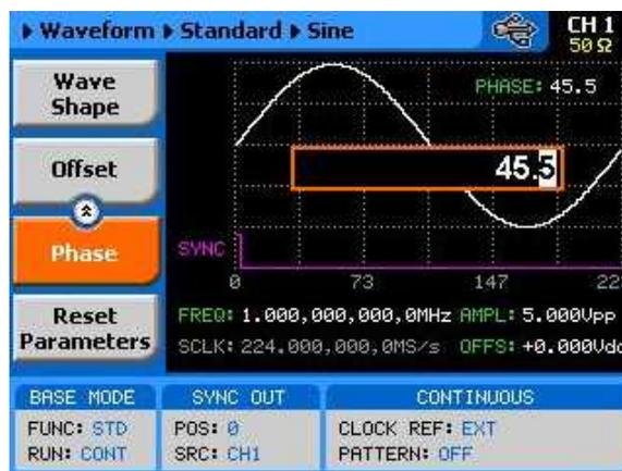
Figure 3-98, Changing the Start Phase on the Sine Waveform
