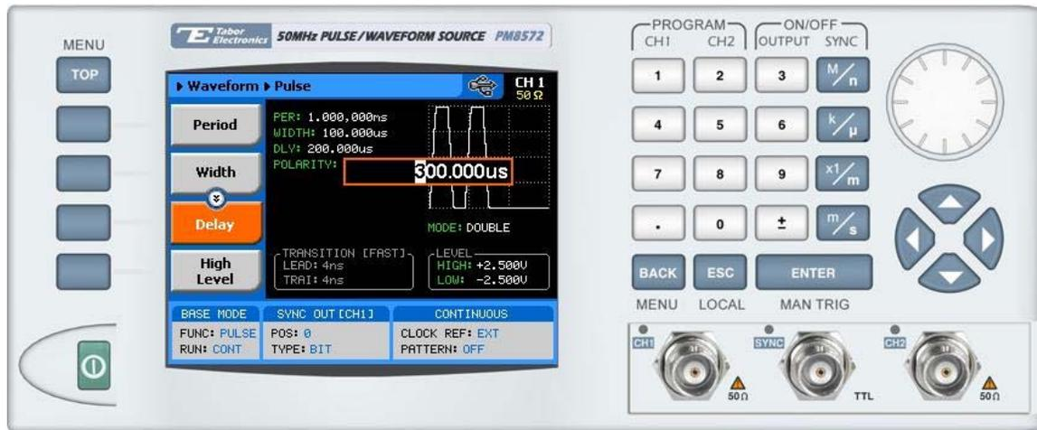
Figure 3-22, Programming the Double Pulse Delay
