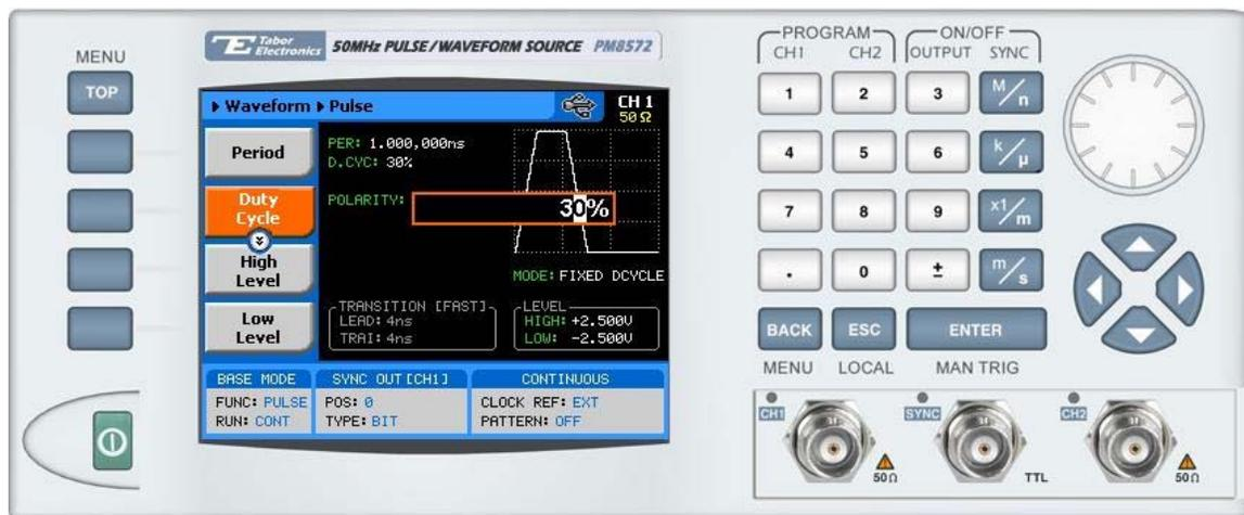
Figure 3-26, Programming the Duty Cycle Parameter
