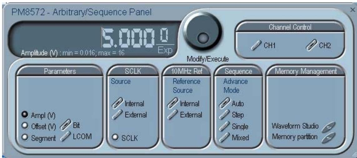
Figure 1-13, ArbConnection Example – Typical Arbitrary & Sequenced Waveforms Panel
