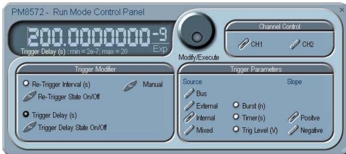
Figure 4-4, the Run Mode Control Panel
