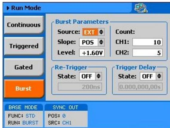
Figure 3-12, Burst Run Mode Parameters
