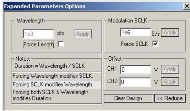
Figure 4-65, the Expanded Parameters Options Dialog Box
