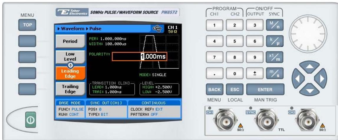
Figure 3-38, Leading Edge Programming Example
