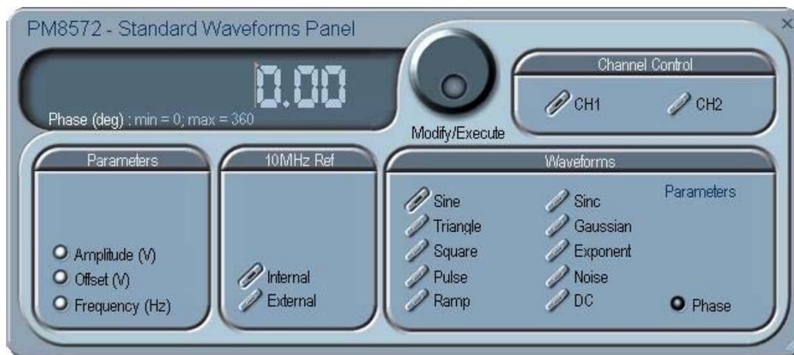
Figure 4-9, the Standard Waveforms Panel
