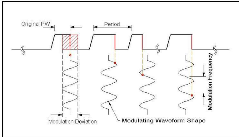
Figure 3-31, Pulse Width Modulation Example
