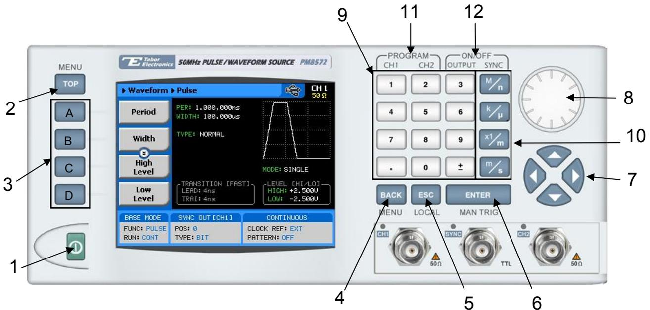
Figure 3-3, PM8572A Front Panel Operation
