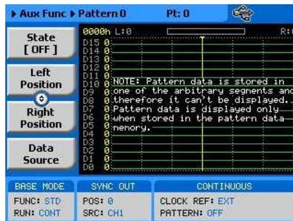
Figure 3-89, Digital Pattern Display while Using the Arbitrary Memory
