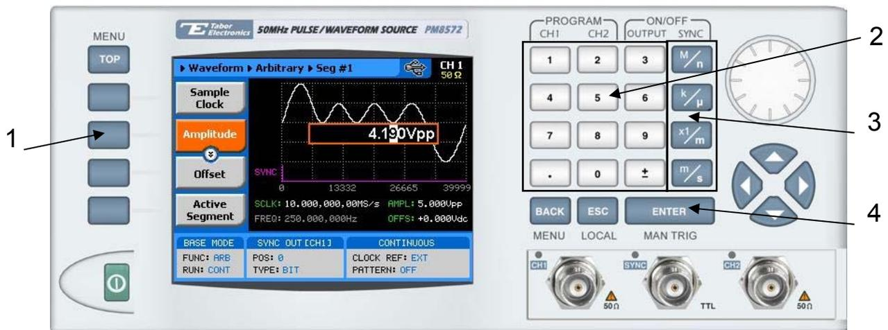
Figure 3-48, Programming Arbitrary Waveform Parameters
