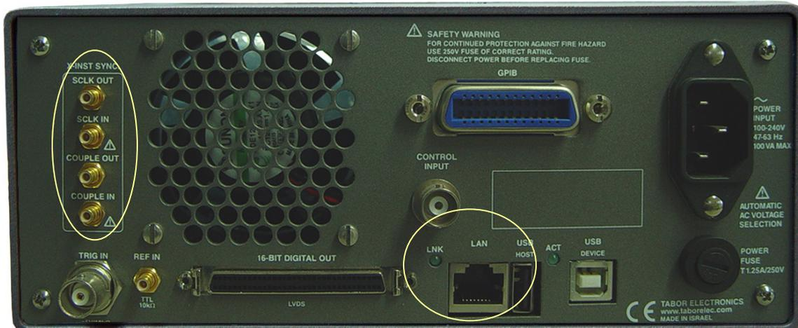
Figure 3-92, Connecting the PM8572A Synchronization Cables
