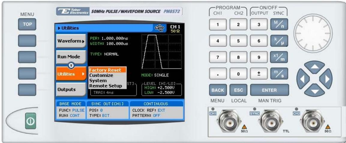
Figure 3-2, Reset PM8572A to Factory Defaults
