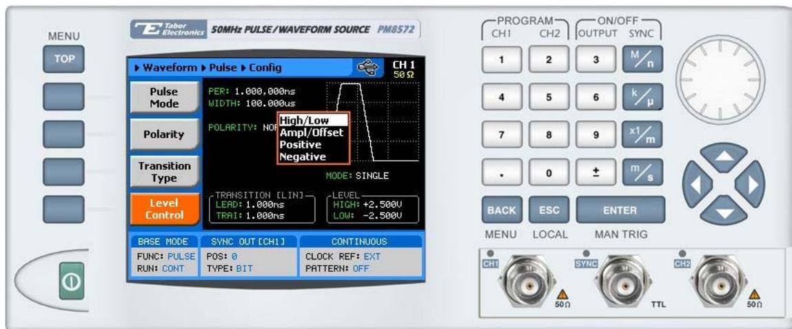
Figure 3-40, the Amplitude Level Control Options
