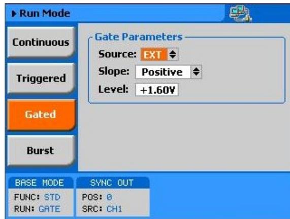
Figure 3-11, Gated Mode Parameters
