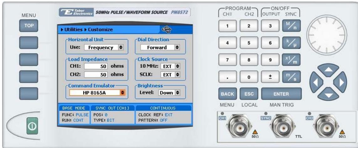
Figure 3-99, Customizing the Output Parameters
