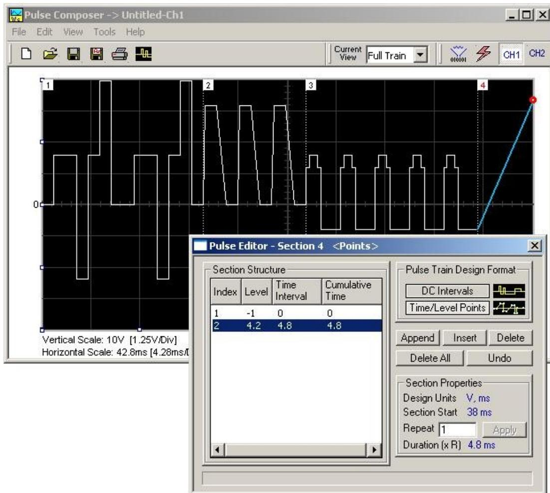
Figure 4-58, Building Section 4 of the Pulse Example
