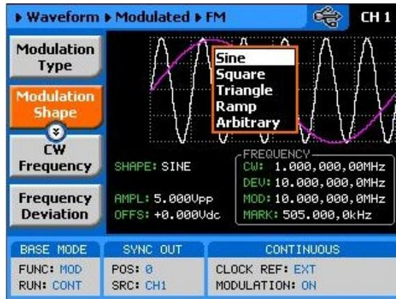
Figure 3-58, Modulation Waveform Shapes
