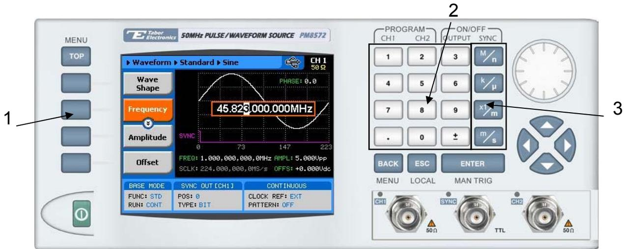
Figure 3-6, Modifying Output Frequency
