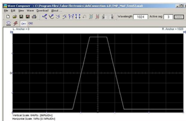
Figure 1-16, Segment 3 Waveform - Pulse
