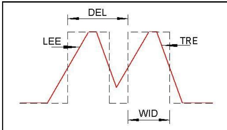
Figure 3-41, Output Waveform with Error 102 (202) Example
