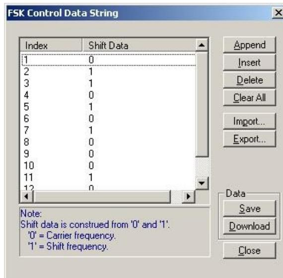
Figure 3-71, FSK Control Data String Example
