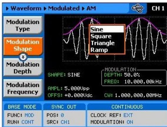
Figure 3-56, Modulating Waveform Shapes
