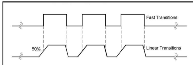
Figure 3-35, Fast and Linear Transitions, Compared
