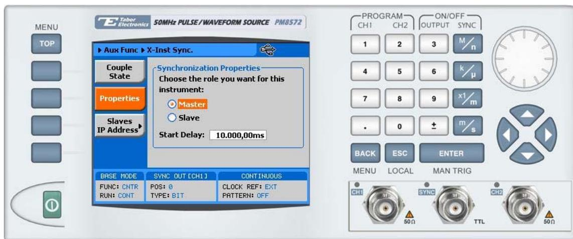
Figure 1-26, Multi-Instruments Synchronization Panel Example
