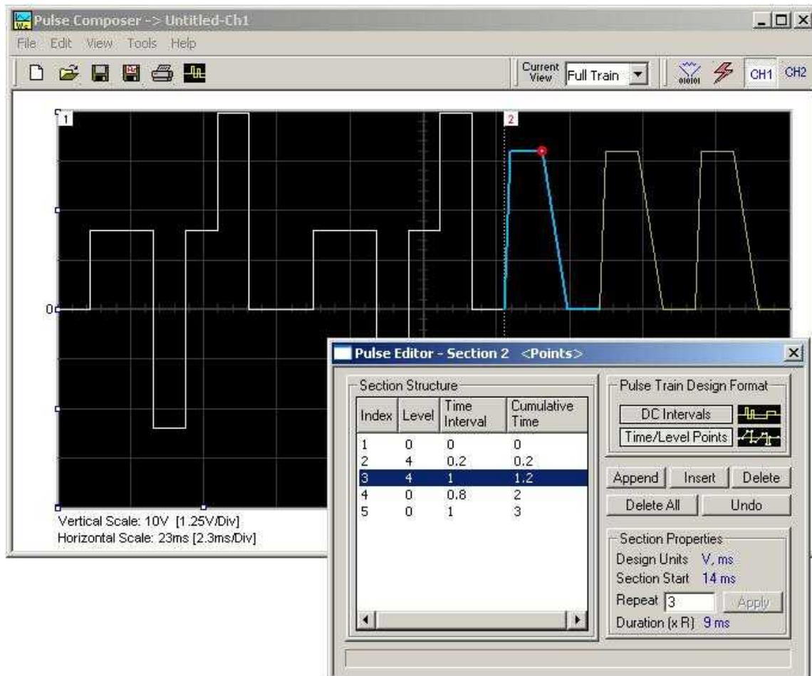
Figure 4-56, Building Section 2 of the Pulse Example
