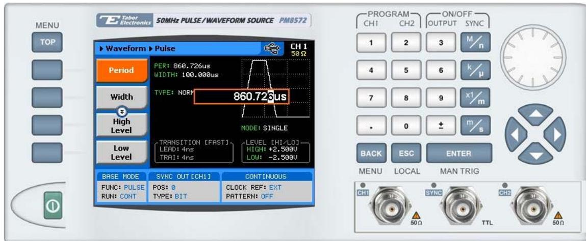
Figure 3-17, Programming the Pulse Period Parameter
