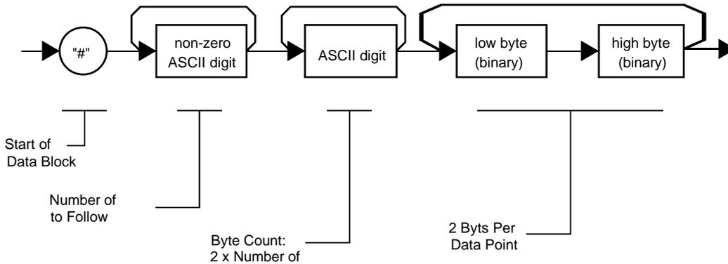
Figure 5-1, Definite Length Arbitrary Block Data Format
