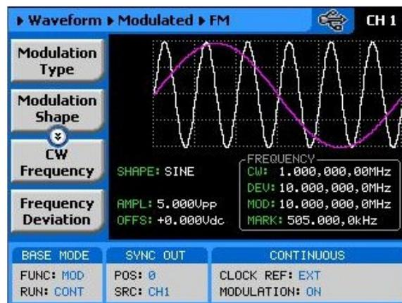
Figure 3-57, FM Modulation Parameters
