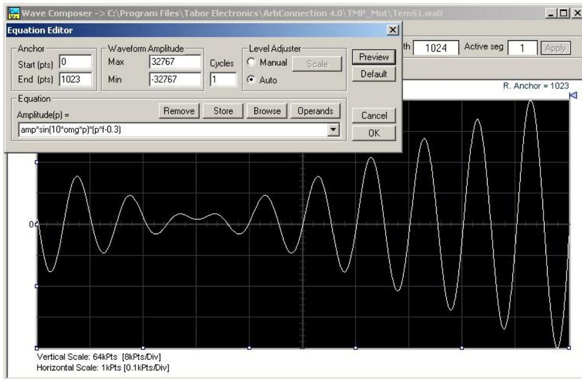
Figure 3-47, the Wave Composer Tool for Generating Arbitrary Waveforms
