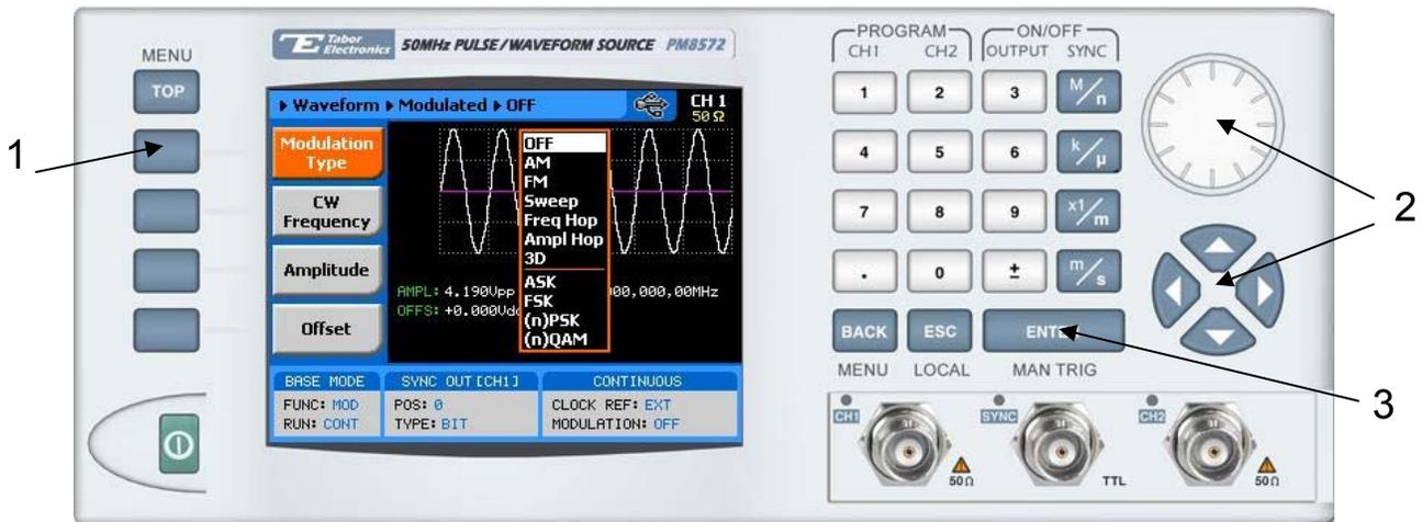
Figure 3-53, Selecting a modulated Waveform
