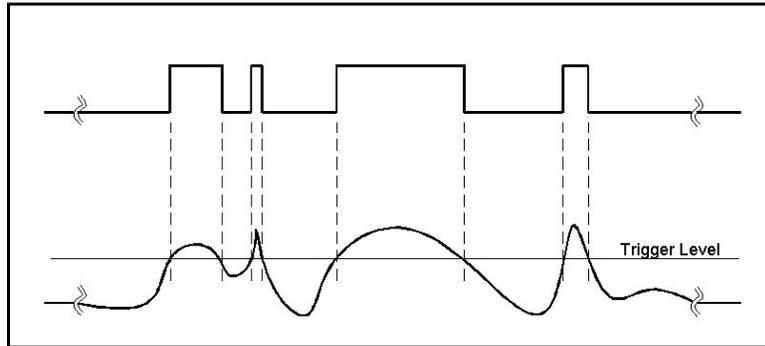
Figure 3-27, External Pulse Width Mode, Positive Slope Example
