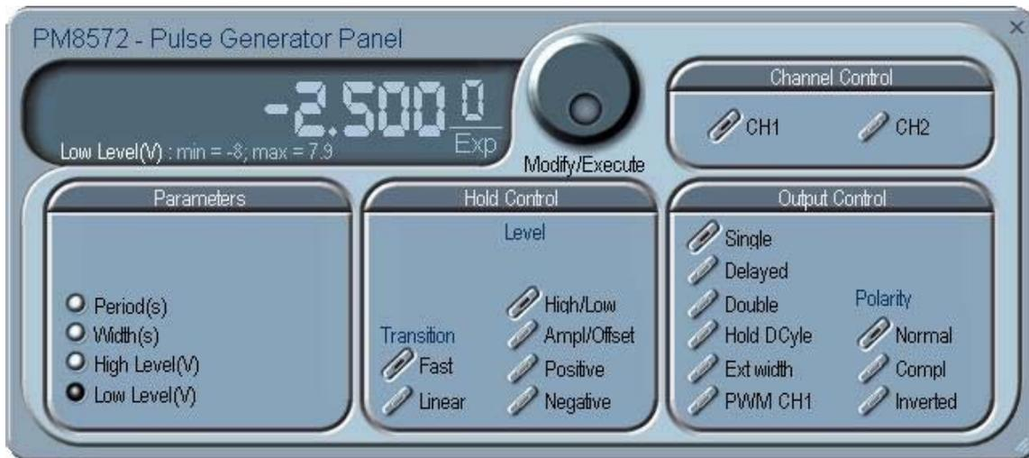
Figure 4-5, the Default Pulse Generator Panel
