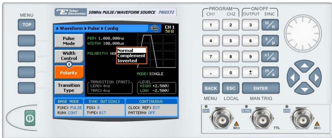
Figure 3-34, Programming the Pulse Polarity
