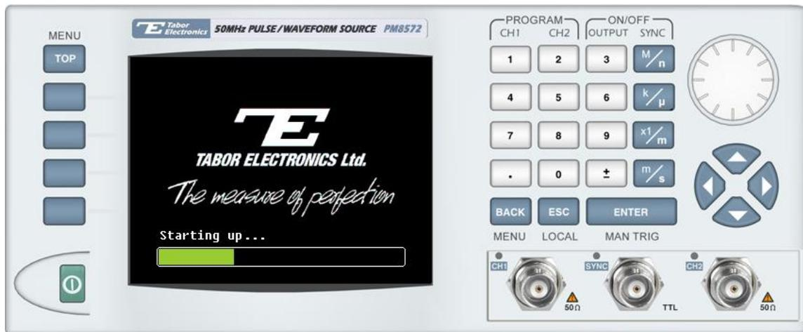
Figure 7-7, Check for Progress Bar Movement
