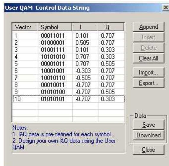
Figure 3-81, User QAM Data Entry Table Example
