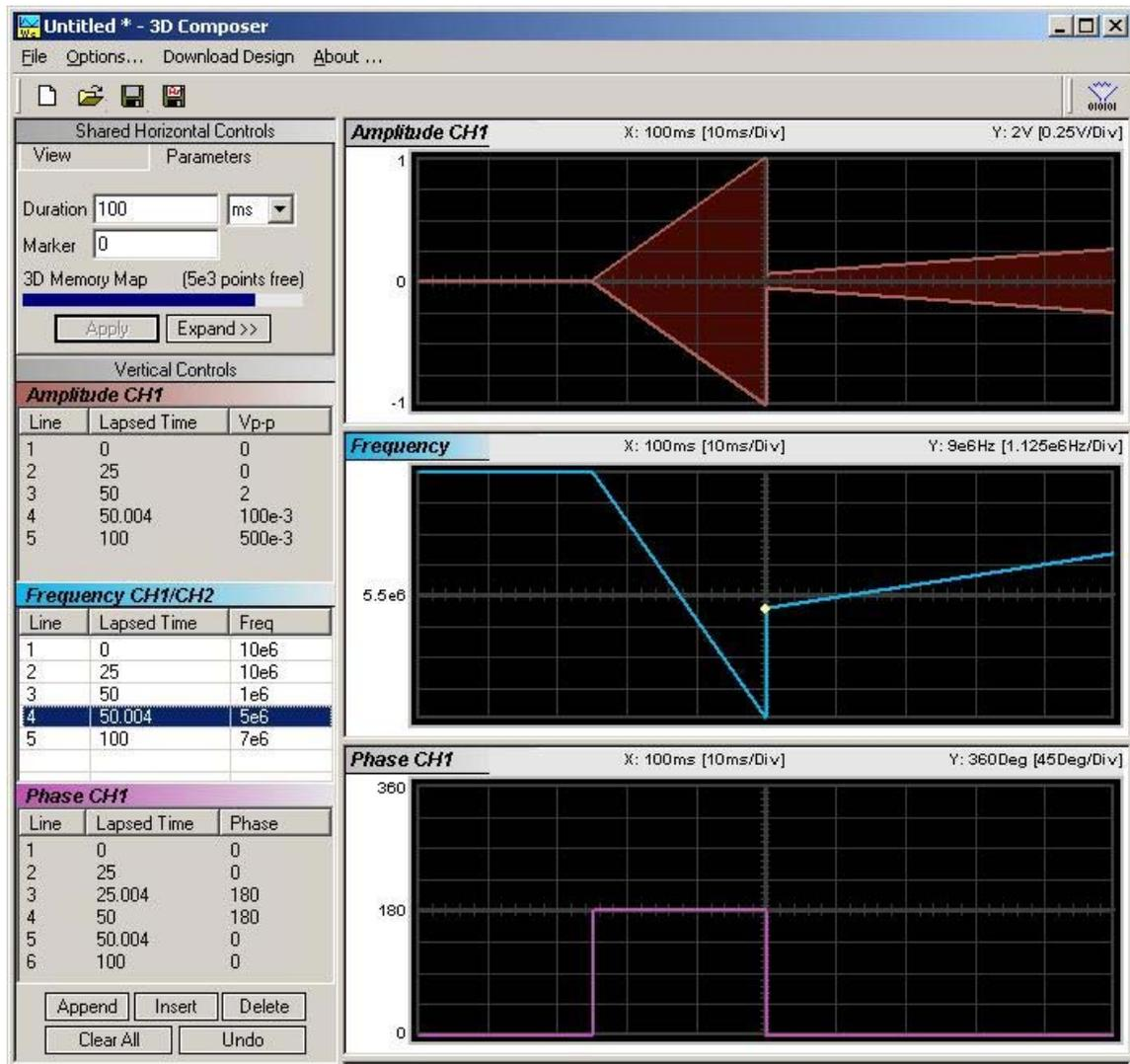
Figure 4-68, 3D Chirp Design Example
