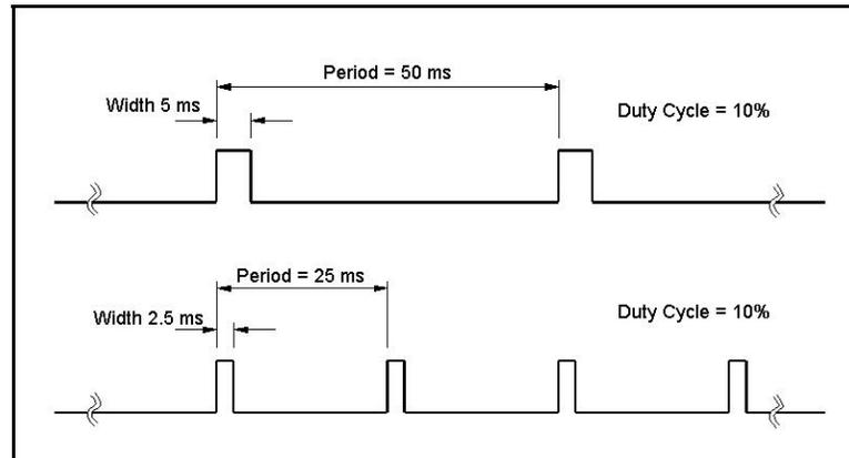
Figure 3-25, Hold Duty Cycle Mode Example
