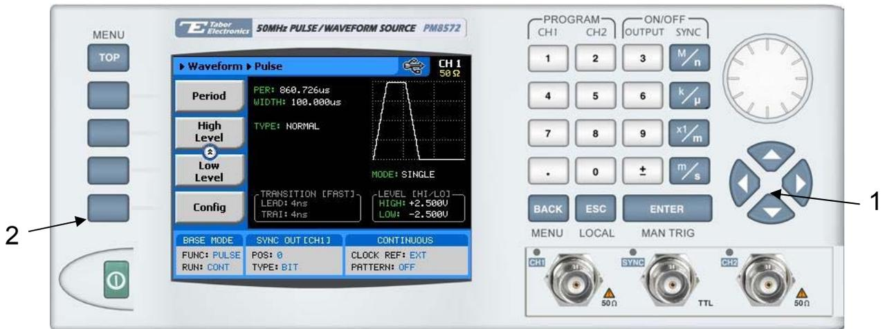
Figure 3-18, Accessing the Pulse Configuration Menus
