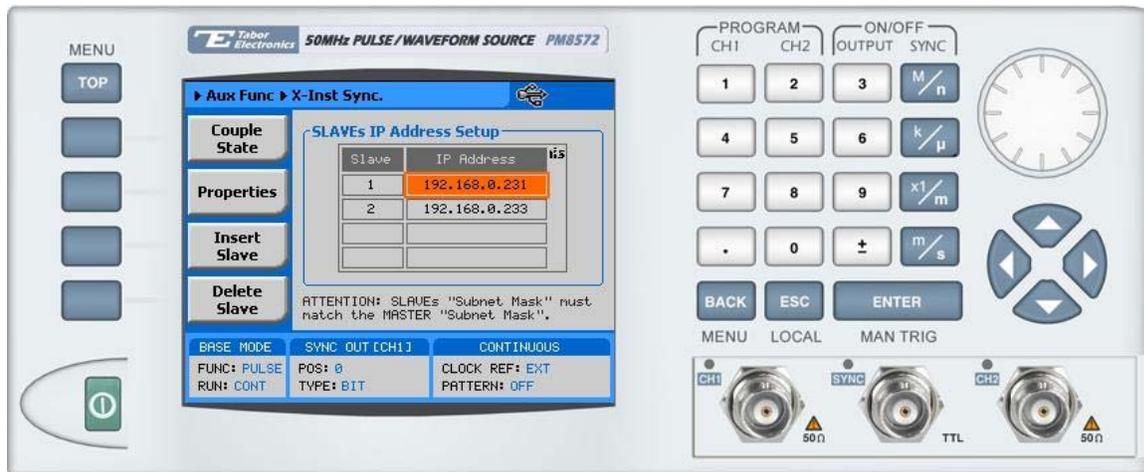
Figure 3-95, Programming Slaves IP Address
