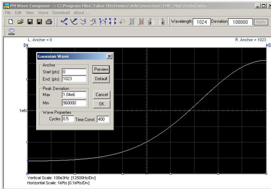
Figure 1-4, ArbConnection – The FM Wave Composer
