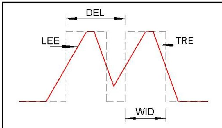
Figure 3-44, Output Waveform with Error 107 (207) Example
