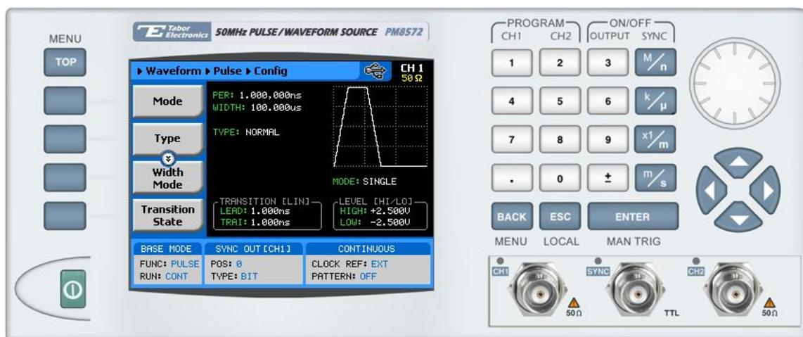
Figure 1-8, PM8572A Pulse Generator Menu Example
