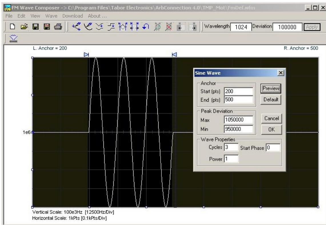
Figure 4-62, Generating Sine Modulation Using the FM Composer
