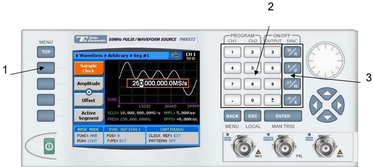
Figure 3-7, Modifying Sample Clock Frequency
