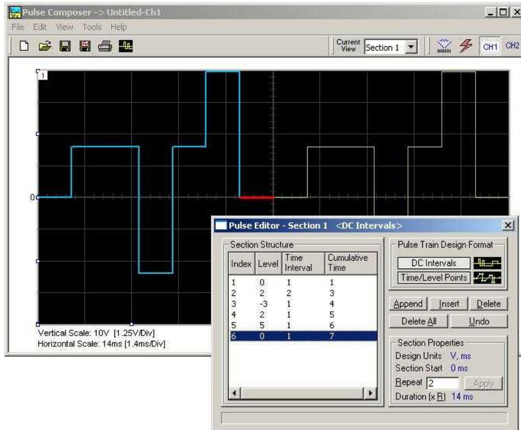
Figure 4-55, Building Section 1 of the Pulse Example
