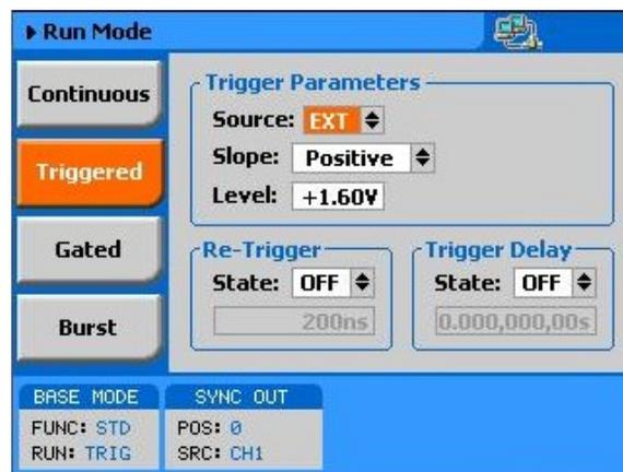
Figure 3-10, Trigger Run Mode Parameters
