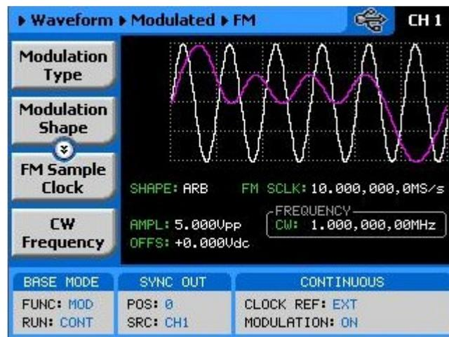
Figure 3-60, Arbitrary Frequency Modulation menus
