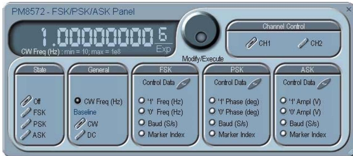
Figure 4-18, the FSK/PSK/ASK Modulation Panel
