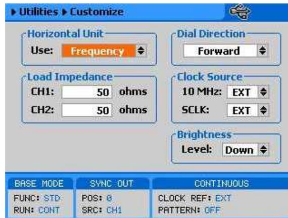
Figure 3-14, Modifying the SCLK and 10MHz Clock Source
