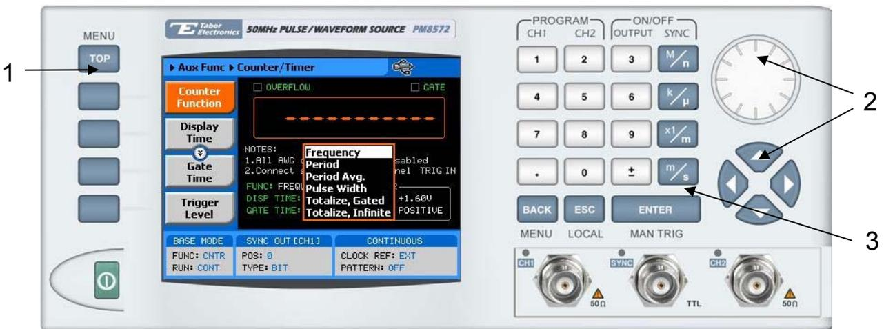
Figure 3-86, Selecting a Counter/Timer Measurement Function
