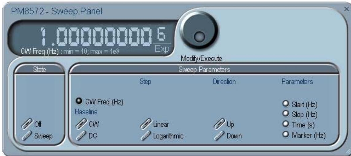
Figure 4-17, the Sweep Modulation Panel
