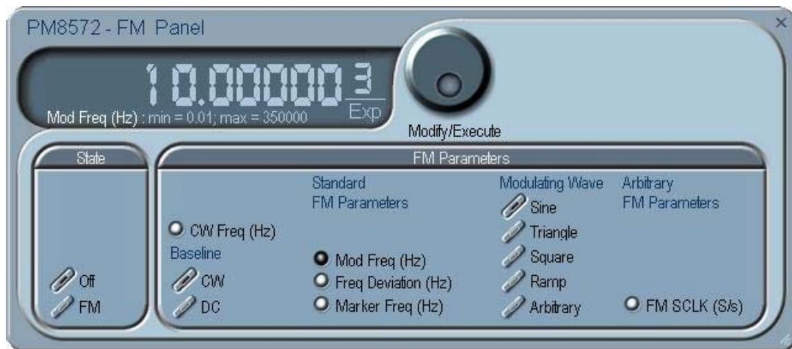
Figure 1-21, ArbConnection Example – FM Modulation Panel
