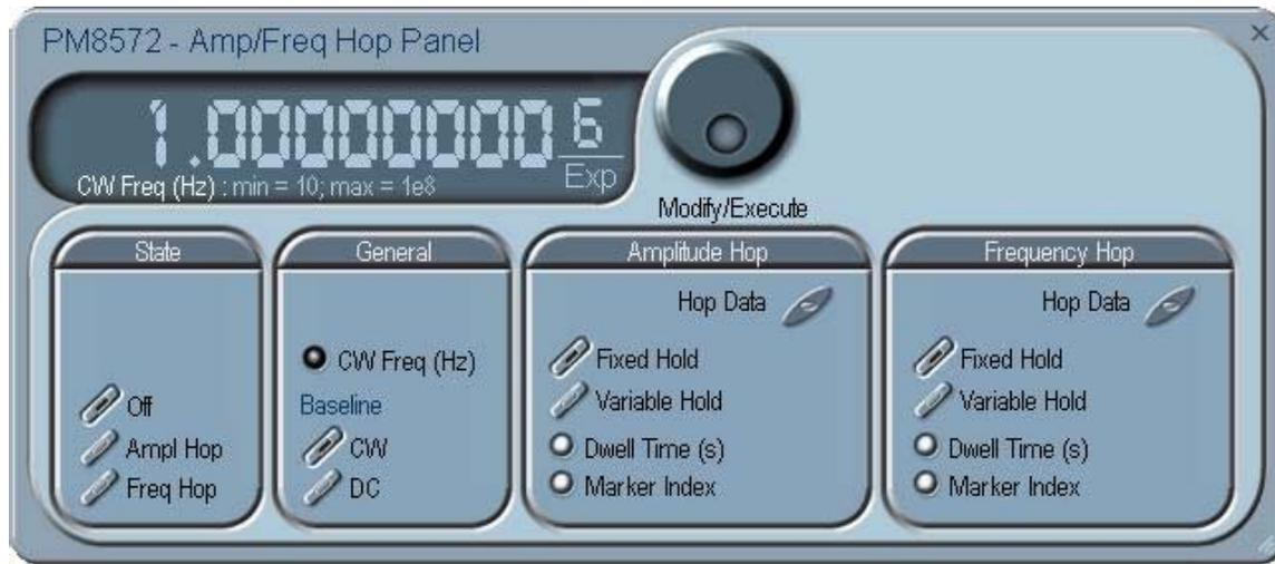
Figure 4-19, the Amp/Freq Hop Panel
