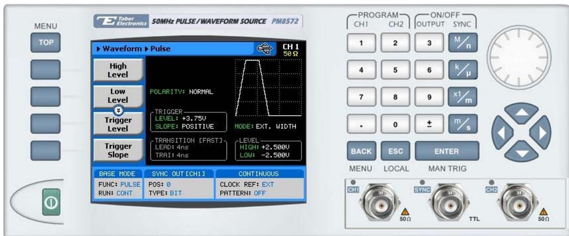
Figure 3-29, External Pulse Width Menus
