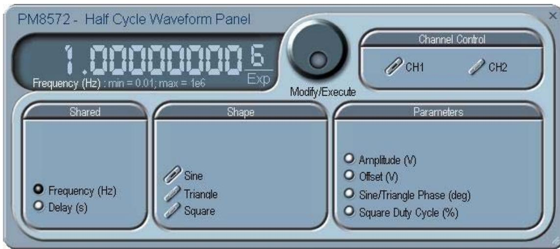
Figure 4-14, the Half Cycle Panel
