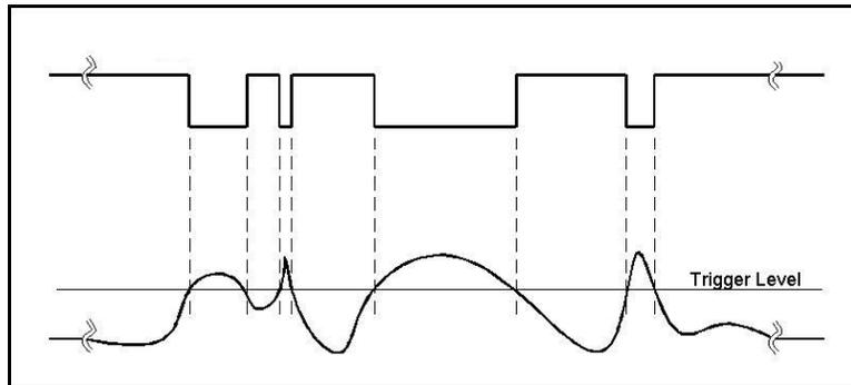
Figure 3-28, External Pulse Width Mode, Negative Slope Example
