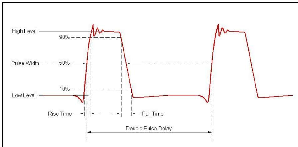
Figure 3-21, Double Pulse Mode
