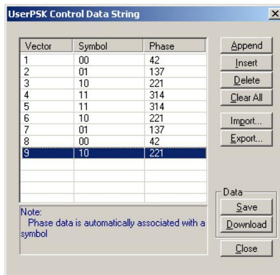
Figure 3-77, User PSK Data Entry Table Example
