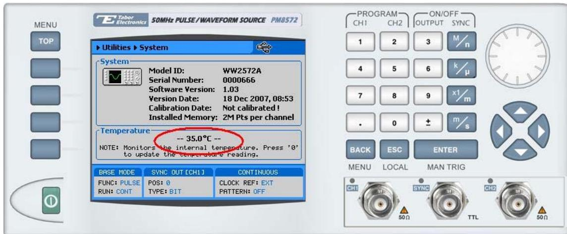
Figure 3-103, Reading the PM8572A Internal Temperature
