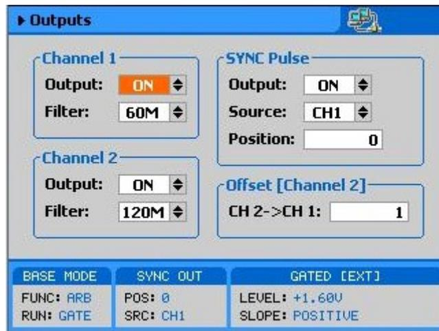
Figure 3-13, SYNC and Filter Parameters
