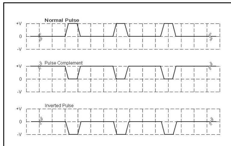
Figure 3-33, Pulse Polarity Options
