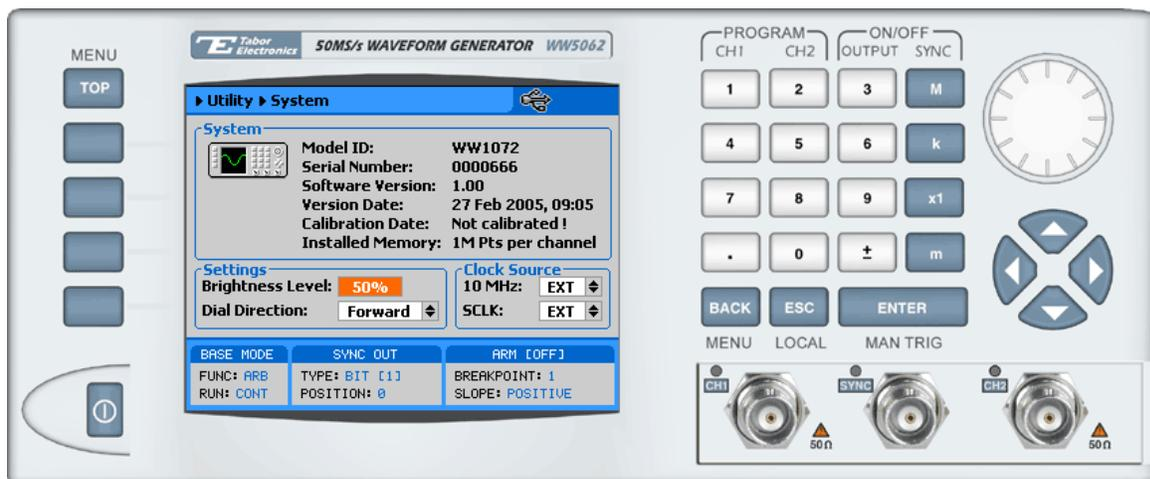
Figure 3-15, Modifying the SCLK and 10MHz Clock Source
