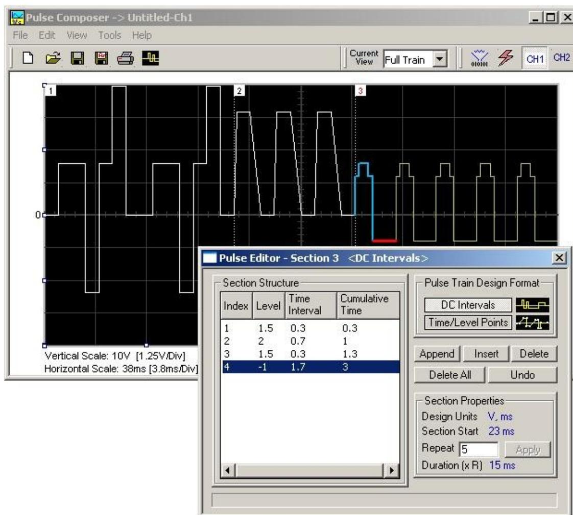
Figure 4-40, Building Section 3 of the Pulse Example
