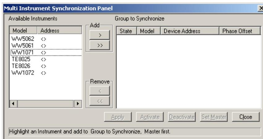
Figure 4-13, The Multi Instruments Synchronization Dialog Box
