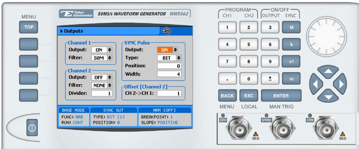
Figure 3-14, SYNC and Filter Parameters
