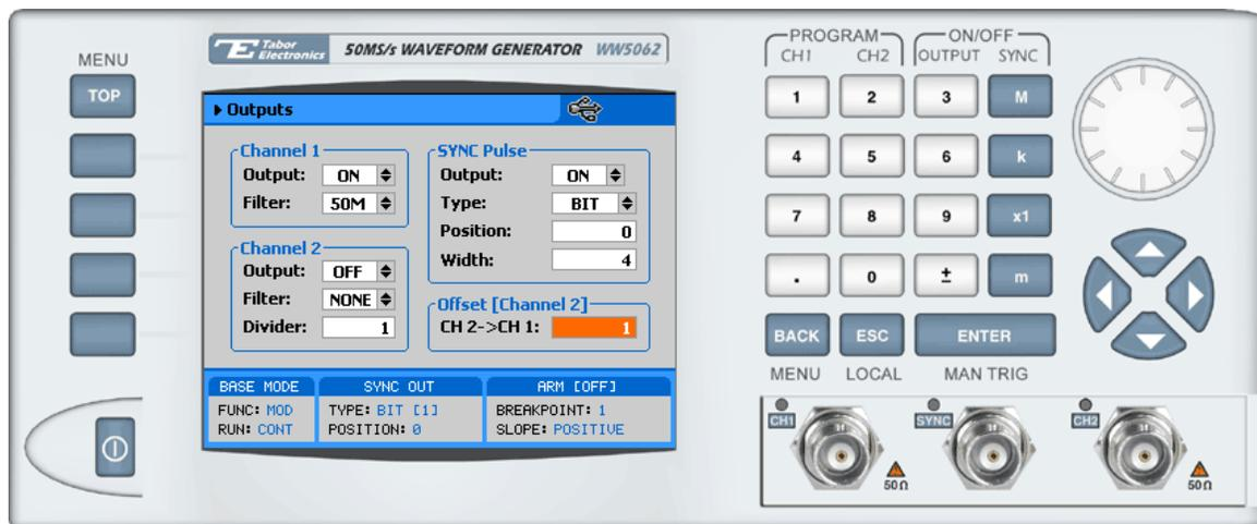
Figure 3-28, Adjusting Phase Offset Between Channels
