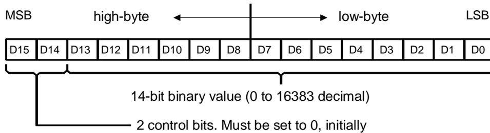
Figure 5-2. 16-bit Initial Waveform Data Point Representation
