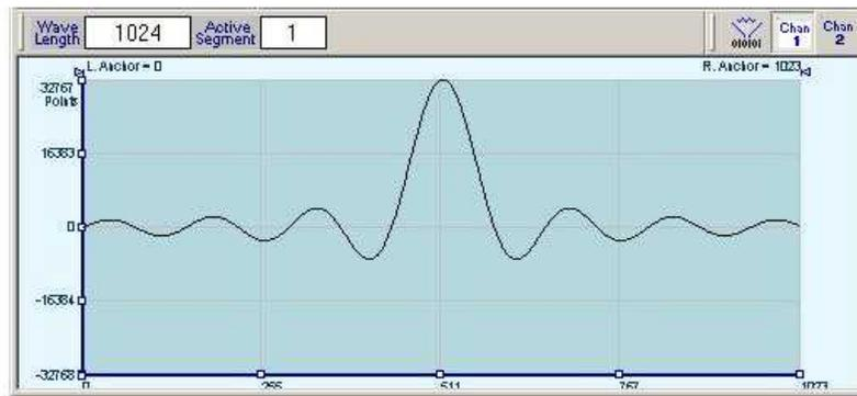
Figure 1-8, Segment 1 – Sin (x)/x Waveform
