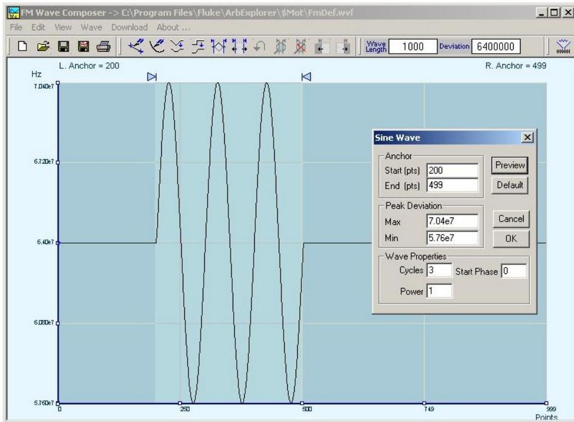
Figure 4-22, Generating Sine Modulation Using the FM Composer
