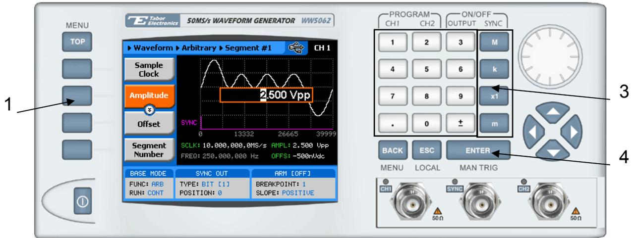
Figure 3-17, Programming Arbitrary Waveform Parameters
