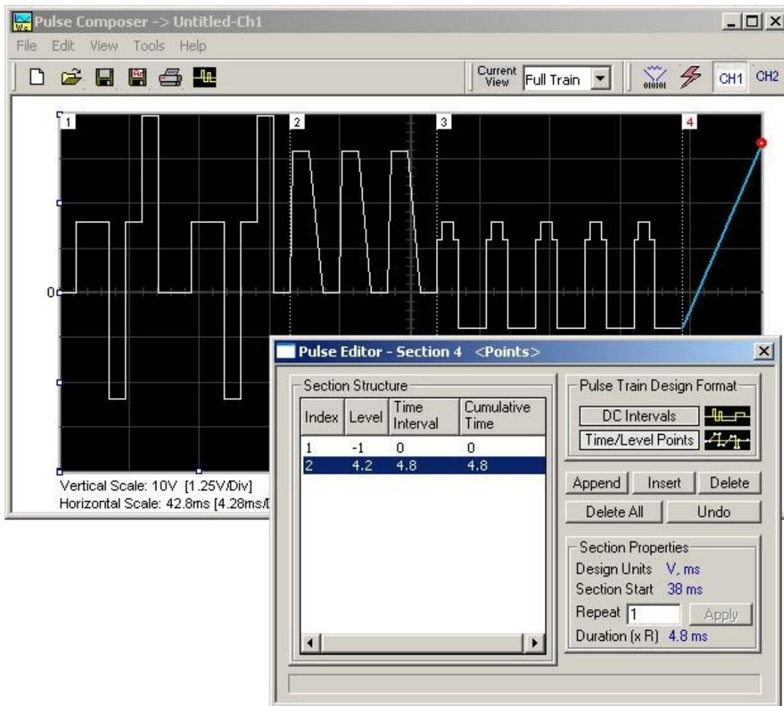
Figure 4-41, Building Section 4 of the Pulse Example
