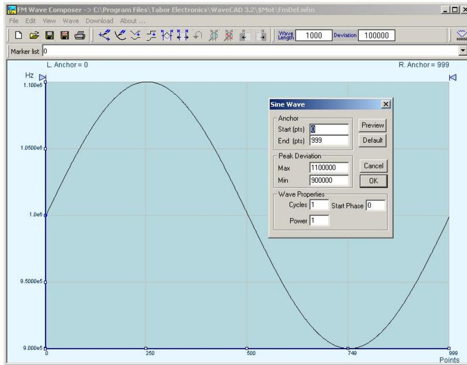
Figure 1-4, ArbConnection – The FM Wave Composer
