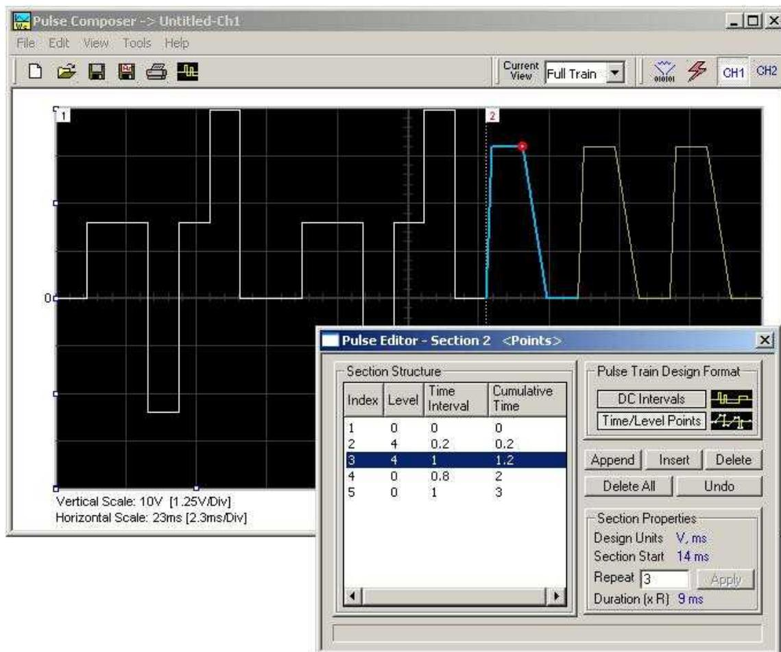
Figure 4-39, Building Section 2 of the Pulse Example
