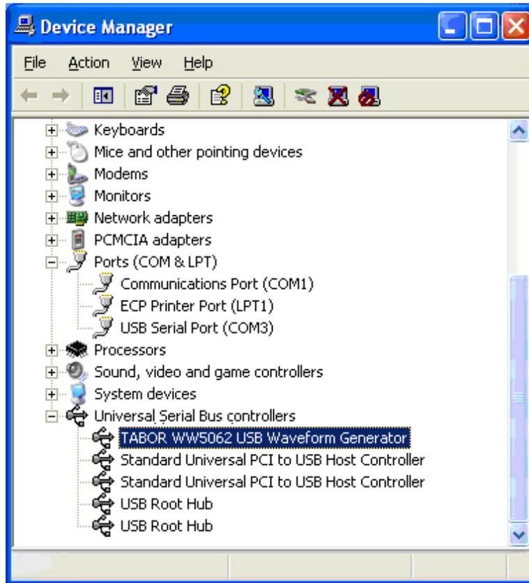
Figure 2-10, Model 5062 Configured for USB Operation
