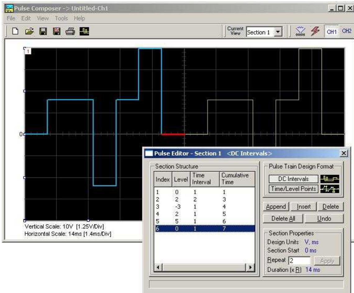
Figure 4-38, Building Section 1 of the Pulse Example
