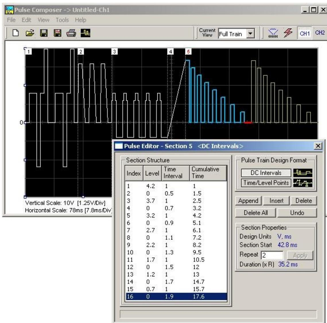
Figure 4-42, Building Section 5 of the Pulse Example
