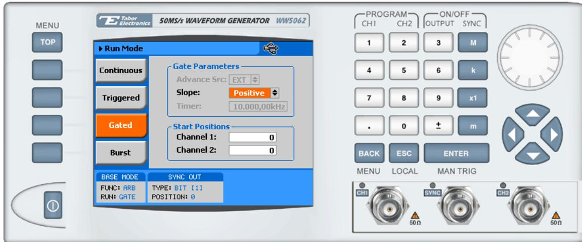
Figure 3-11, Gated Mode Parameters
