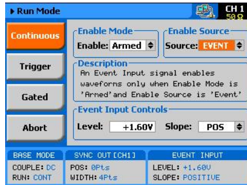
Figure 3-11, Typical Continuous Run Mode Display with the Abort Soft Key
