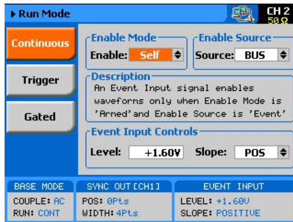
Figure 3-8, The Typical Run Mode Display (Continuous Mode Shown)
