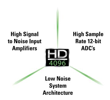
Teledyne LeCroy HDO high definition oscilloscopes use unique HD4096 technology to provide superior and uncompromised measurement performance:
