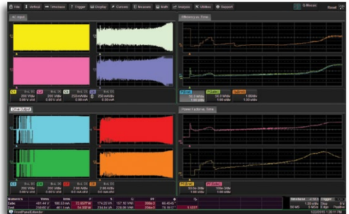
This 480V drive has 10 second acquisitions for the AC Input and Drive Output (on the left) and on the right are shown power, efficiency and power factor Waveforms over time.
