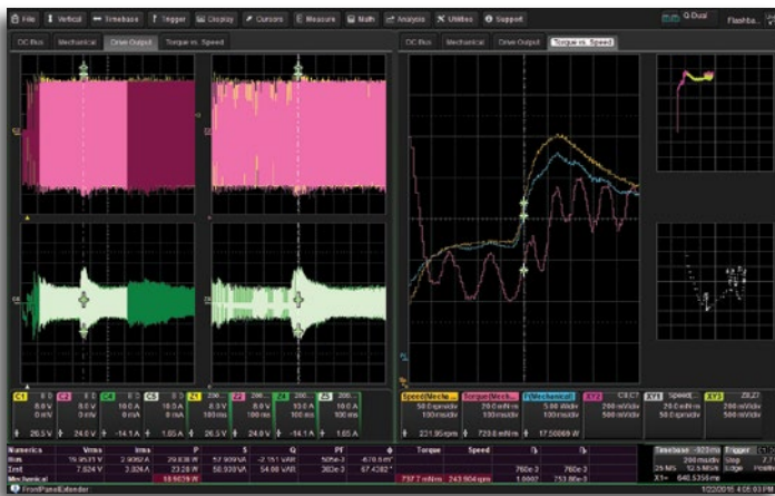
This two second capture shows the drive output waveforms on the left and the Torque, Speed and Mechanical Power Waveform per-cycle values over time are shown to the right.
