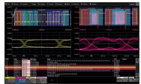
*WaveRunner 8000 combines Serial Bus Trigger, Decode, Measure/Graph, and now also Eye Diagrams*
