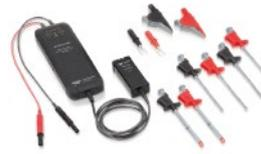
Low cost active differential probes are intended for measuring higher voltages. The differential techniques employed permit measurements to be taken at two points in a circuit without reference to the ground, allowing the oscilloscope to be safely grounded without the use of opto-isolators or isolating transformers.
