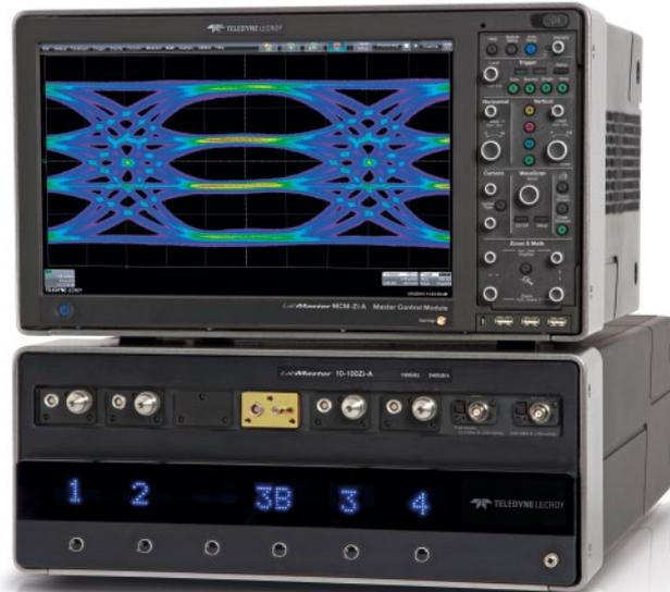
The LabMaster 10 Zi-A series of real-time oscilloscopes boasts the world's highest bandwidth and fastest sampling rate at 100 GHz and 240 GS/s. This world-leading performance is key to acquiring, analyzing and understanding the fastest phenomena found in R&D labs, where engineers are working on next-generation communication systems, high bandwidth electrical components and fundamental scientific research.
