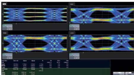
*PAM4 signaling is seen as the next step in the evolution of serial data signal formats, allowing two bits of information to be transmitted per UI rather than one.*
