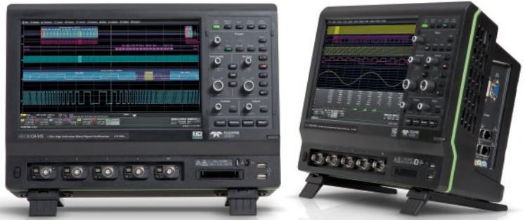
HDO6000 uses Teledyne LeCroy's HD4096 high definition true 12-bit technology, long memory, a compact form factor, 12.1" touch screen display, powerful measurement and analysis tools, and mixed signal capability. It is the ideal oscilloscope for circuit validation, system debug and waveform analysis.
