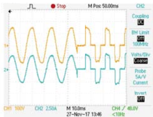
Linear CC mode, UPS Sine to Square Waveform
