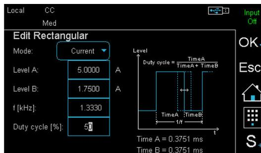
With the PWM function, the switching frequency and the duty cycle can be set for the two amplitude values in manual operation.
