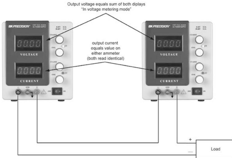
Figure 8 - Connecting Two Power Supplies in Series
