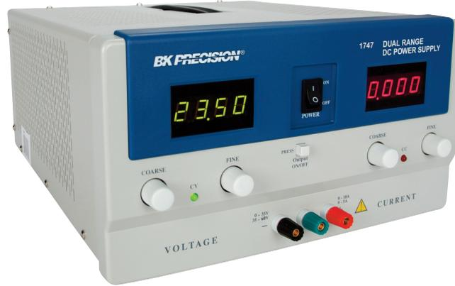
B&K Precision's models 1737 and 1747 are general purpose dual range DC power sources. These power supplies can output higher voltage at a lower current range or more current at a lower voltage range. Two 4-digit LED displays continuously monitor the output voltage and current. The power supplies can be operated locally from the front panel or remotely through the RS-232 interface.
