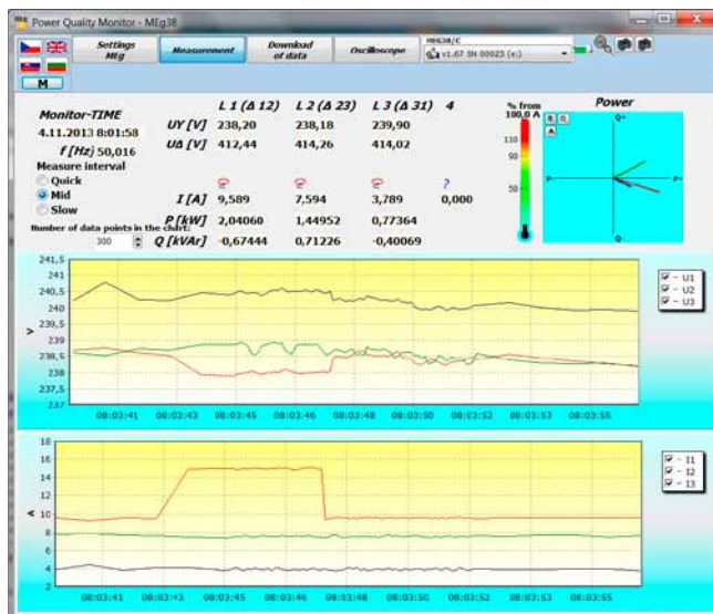
Fig. 25: Measurement and check of connected quantities, course of RMS values
