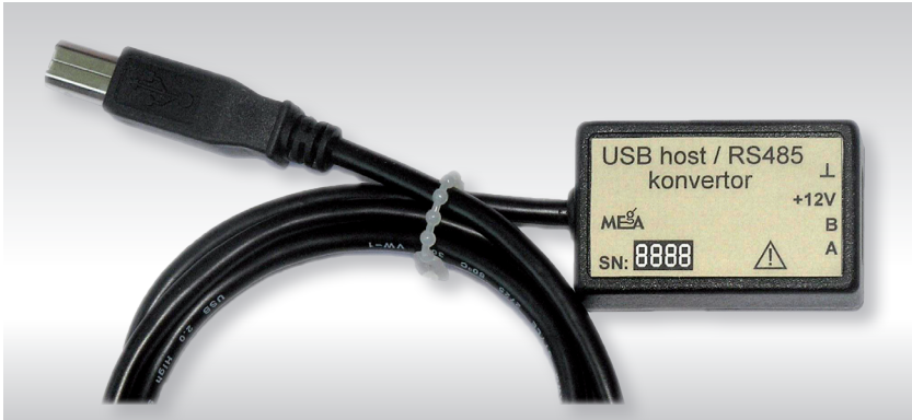
Fig. 1: USBhost/RS485 converter in version for MEg40+ and MEg202.2
