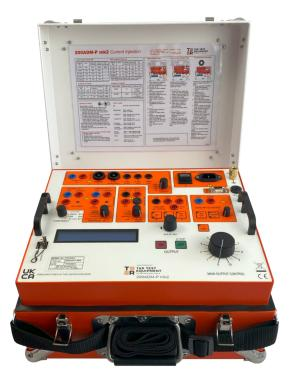
The 200ADM-P Mk2 is a current injection system with a wide range of advanced features including phase shift, data storage and total harmonic analysis.
