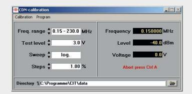
When selecting **<Self-calibration>**, the test equipment will perform a self-calibration. In this case, the output of the signal generator must be connected to the input of the voltmeter.
