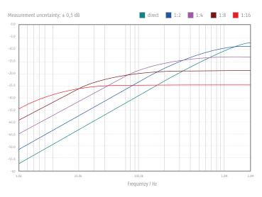
Insertin loss when using the matching transformer MT-1. The selection of the ration in dependence of the frequency can be optimized by automatic software control via LAN or UB-interface.
