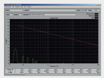
Open the Magnetic field measurement window for spectrum analyzer measurements. Perform a single or continuous measurement. Perform test according to predefined standards.
