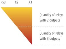
RSU 2223 = 2 relays with 2 outputs and 2 relays with 3 outputs
