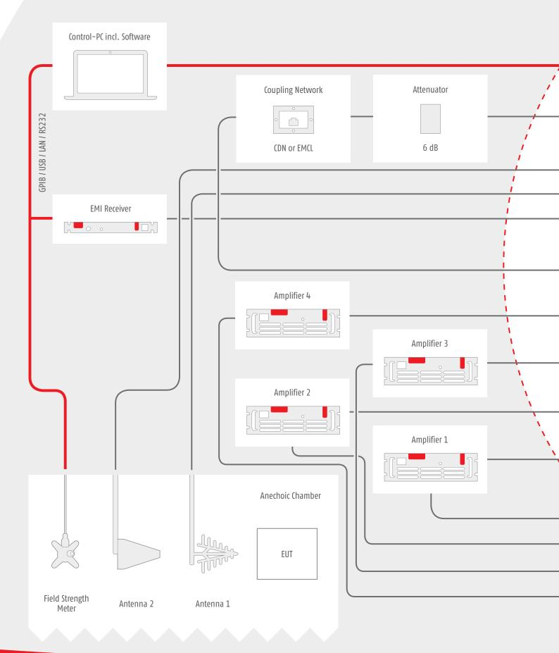
EXAMPLE OF A TEST SYSTEM SETUP WITH ECU-3/-6
