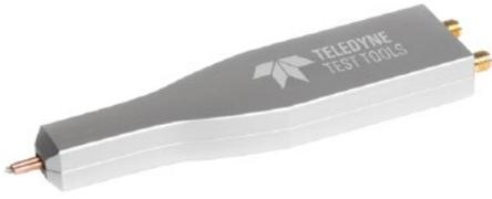
The high precision differential TDR Probe **T3SP-DPROBE** provides an 18 GHz, high performance solution for TDR circuit board impedance characterization and high-speed electrical signal analysis applications. The ergonomic and robust case design providing best ratio of thickness and width. The robust measuring tips guarantee a long life and high repeatability of the measurements.
