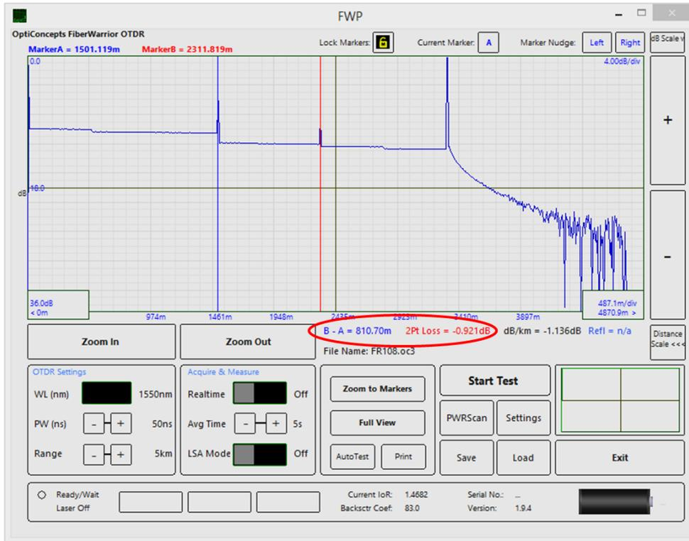
Figure 14 Measurement and 2-Point Loss Measurement
