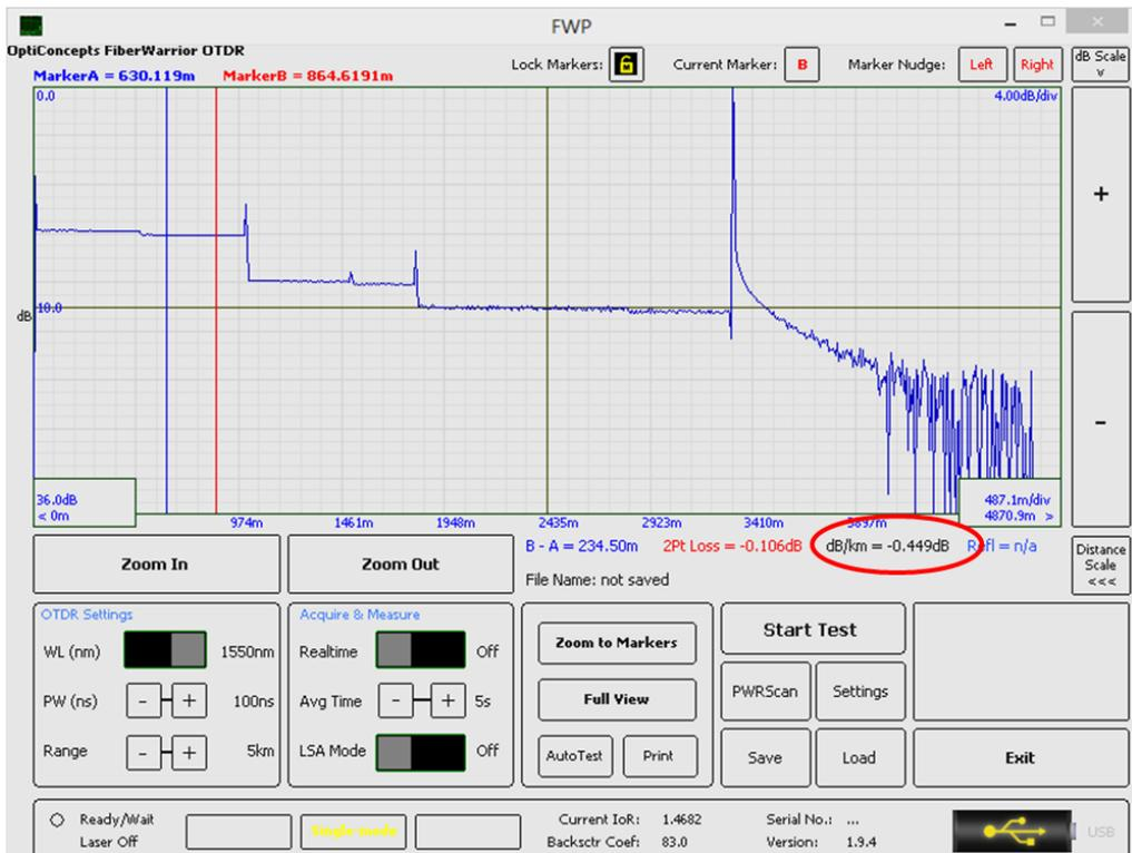
Figure 15 dB/km Measurement
