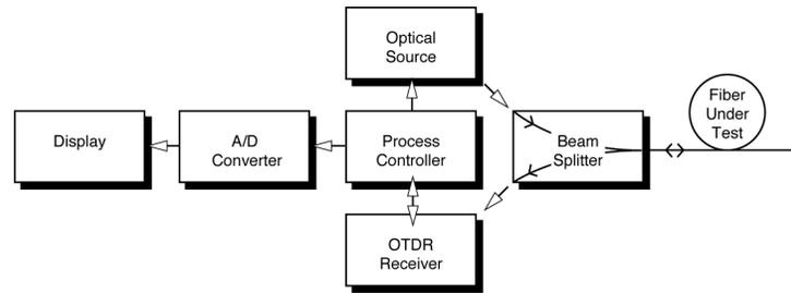
**Figure 2 Basic OTDR Block Diagram**
