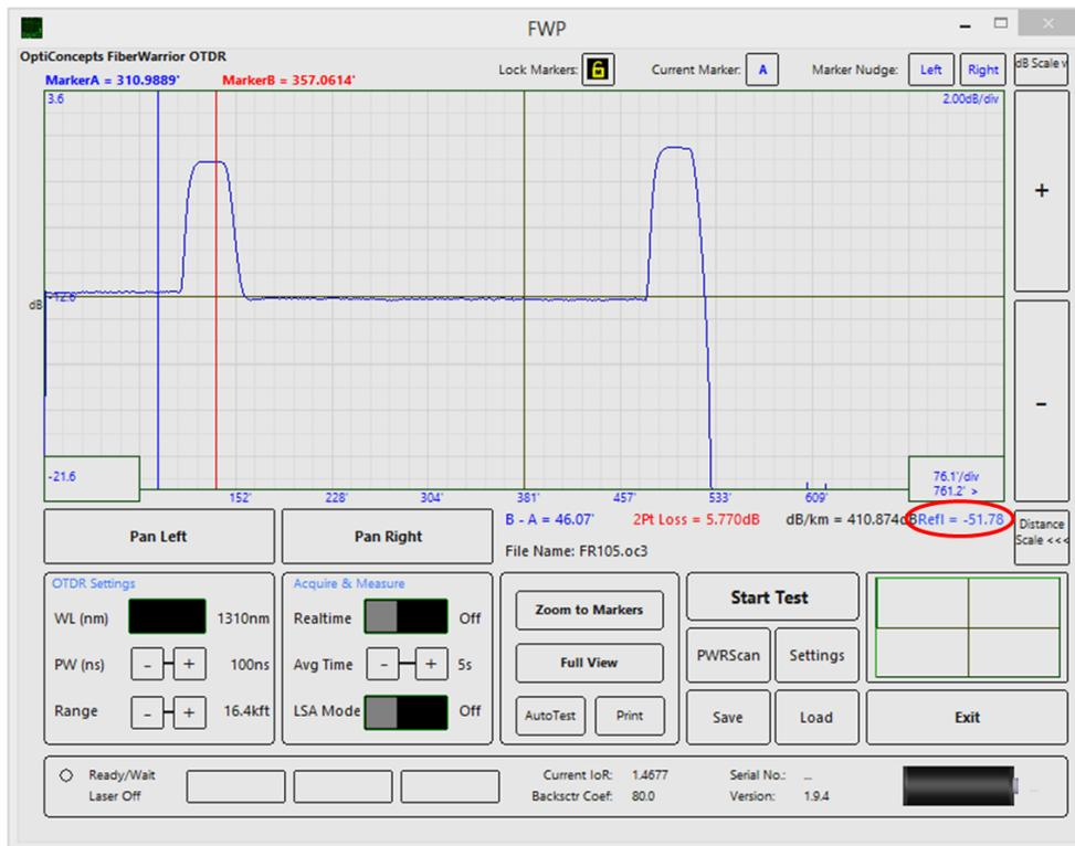
Figure 16 Reflectance Measurement
