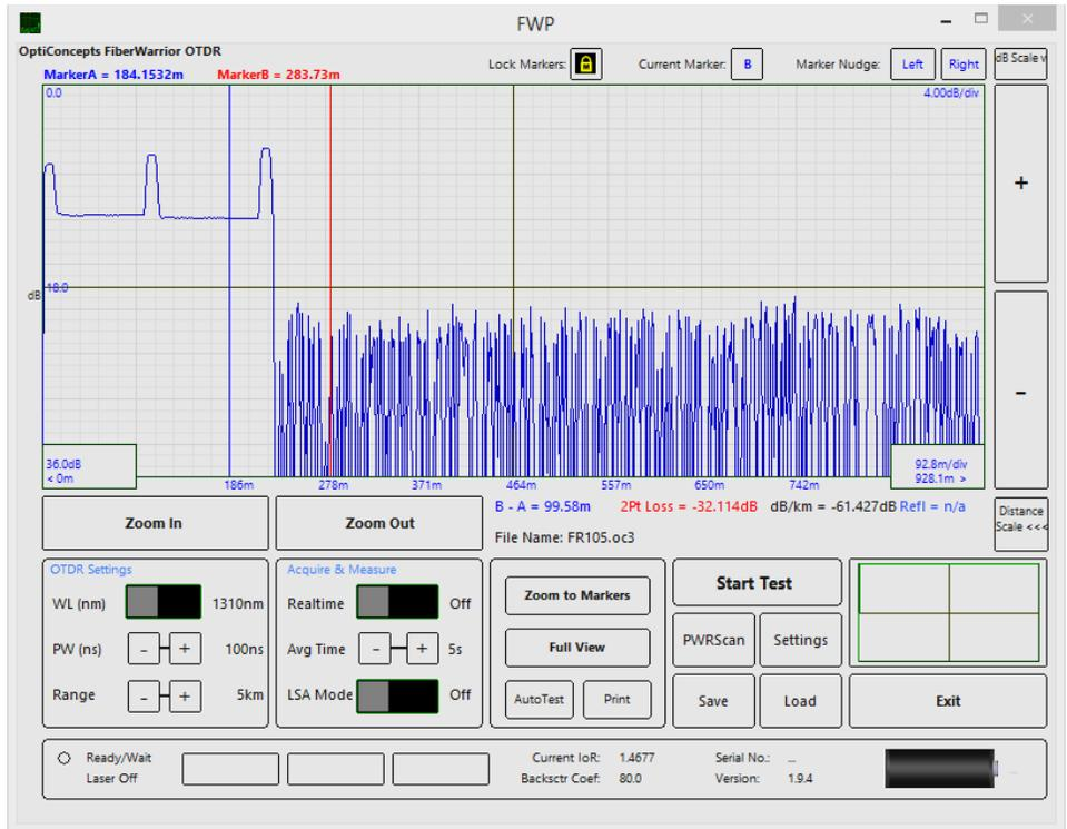
Figure 1 Typical Fiber Trace
