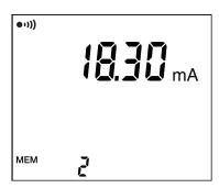
Once the measurement has stabilized, you can press the HOLD key to freeze it and/or MEM to record it.
