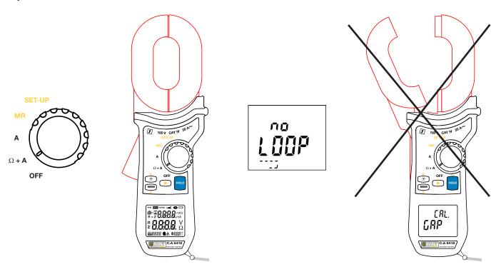
If the instrument fails to make the adjustment, it reports an error by displaying **Err. CAL**. If this happens, switch the instrument off, check that the air gaps are clean, then switch the instrument back on.
