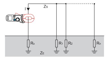
The earth electrode to be measured, Rx, is in parallel with the others via earth  $Z_E$  and guard wire  $Z_S$ .
