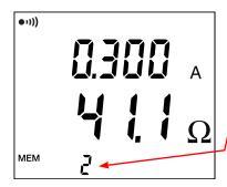
The measurement is recorded in the memory slot of which the number is displayed (here slot number 2).
