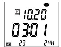
Use the ▲ and ▼ keys to scroll through all of the recorded measurements.
