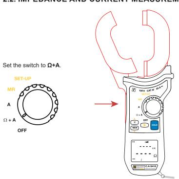
Press the trigger to open the jaws of the clamp and clamp a conductor that is part of the loop to be measured.
