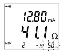
The alarm part of the display unit blinks and the instrument emits a continuous audible signal.
