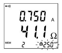
If you set alarms on both the impedance and the current and both alarm thresholds are exceeded, it is the alarm on the current that has priority.
