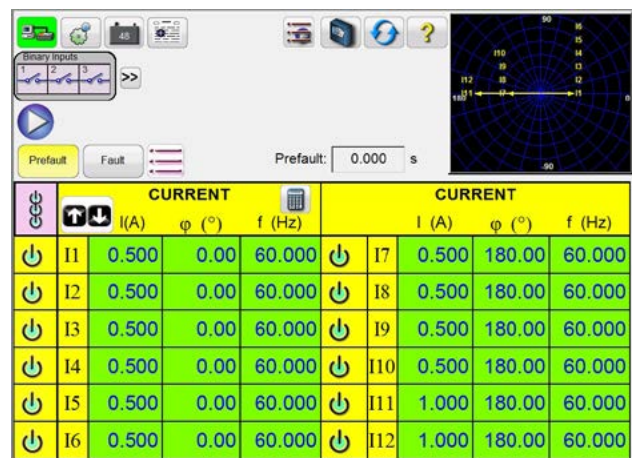
12 Currents Simulating a Bus Differential Scheme
