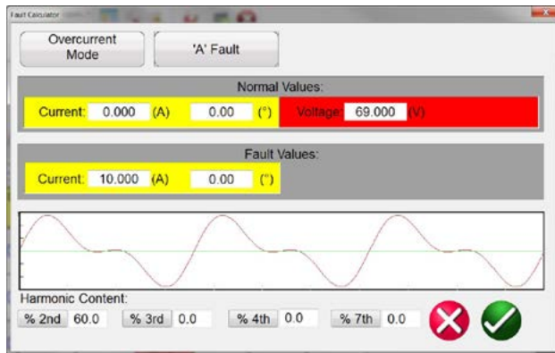
Fault Calculator Displays Harmonic Waveforms
