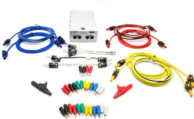
**The HVA Current Module** provides two 25 A sources at 150 VA each. When both sources are connected in parallel, 50 A at 300 VA continuous power is produced. Transient mode extends power and range up to 90 A at 300 VA for 30 seconds. DC output is 50 A.
