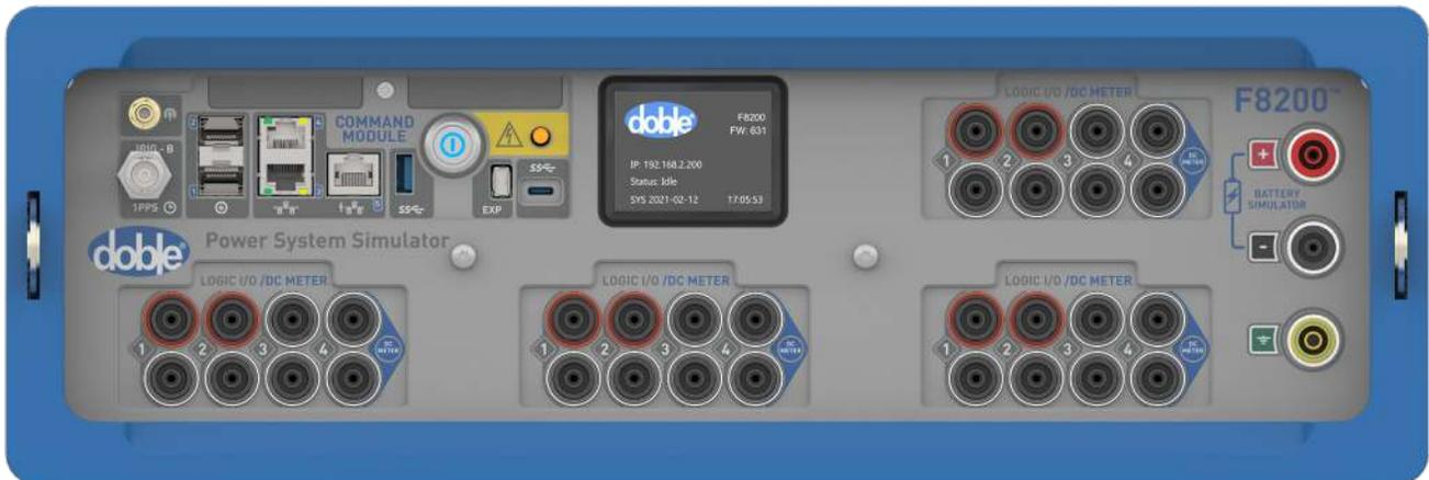
Drive this F8200 with your existing Protection Suite and RTS test procedures. The state-of-the-art digital componentry enables powerful simulations that include the necessary communication functions for testing modern protection schemes including architectures based on the IEC 61850 standard.
