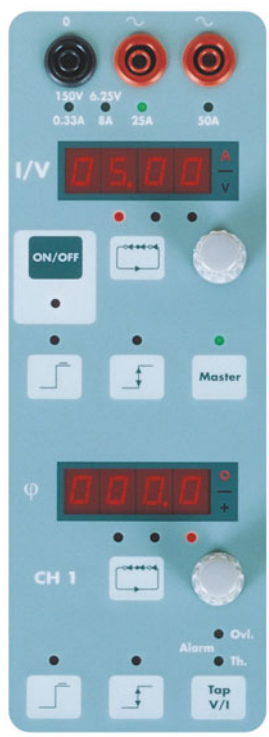
Current / voltage channel
